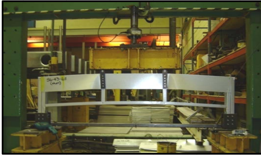
Figure 5.1 Uplift Load Case - Buckling Failure of Web Section (6' Assemblies)
