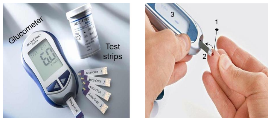
Figure 1.1: Finger pricking methodology for BGL testing using Glucometer devices. 1. Lancet needle, 2. Transfer the extracted blood sample to test strip, and 3. Processing and displaying the resulting BGL on the screen.
