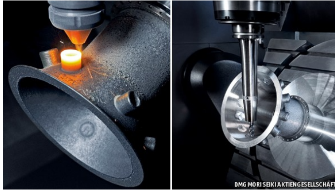
Figure 2.2: Hybrid manufacturing system, where DED and machining processes are combined in one manufacturing system [1]
