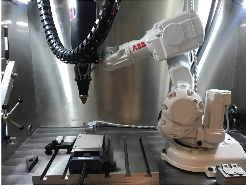
Figure 3.14: DED experimental setup used for model validation
