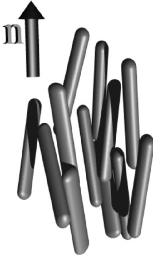
Figure 2.4: The director (a unit vector) of a nematic calamitic liquid crystal is represented by \mathbf{n} [8].
