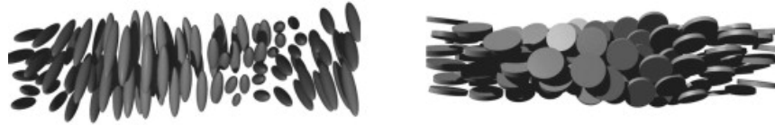
Figure 2.10: Molecular arrangements in a chiral nematic (“cholesteric”) phase [8] formed by calamitic (left) and discotic (right) mesogens. Note that the drawing is not to scale - in a real system the degree of order would be lower and the pitch of helix-like rotation would be significantly longer.
