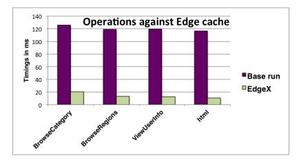
Figure 6.4: Comparison in latency for RUBiS workload operations executed at the Edge site.
