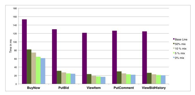
Figure 6.5: Impact on latency of VC initiated web operations when certain percentage of items are equally accessed from edge CT too.
