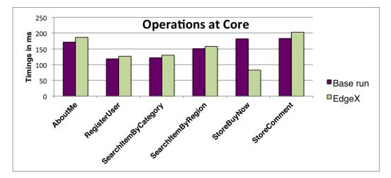
Figure 6.2: Comparision of latency for RUBiS workload operations executed at the Core site.
