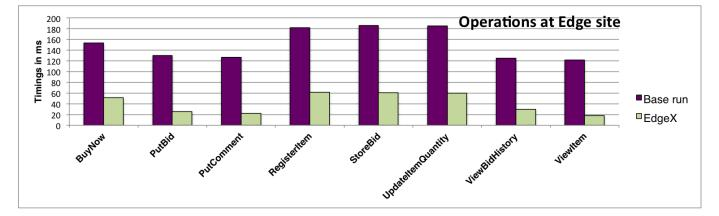
Figure 6.3: Comparison in latency for RUBiS workload operations executed at the Edge site.
