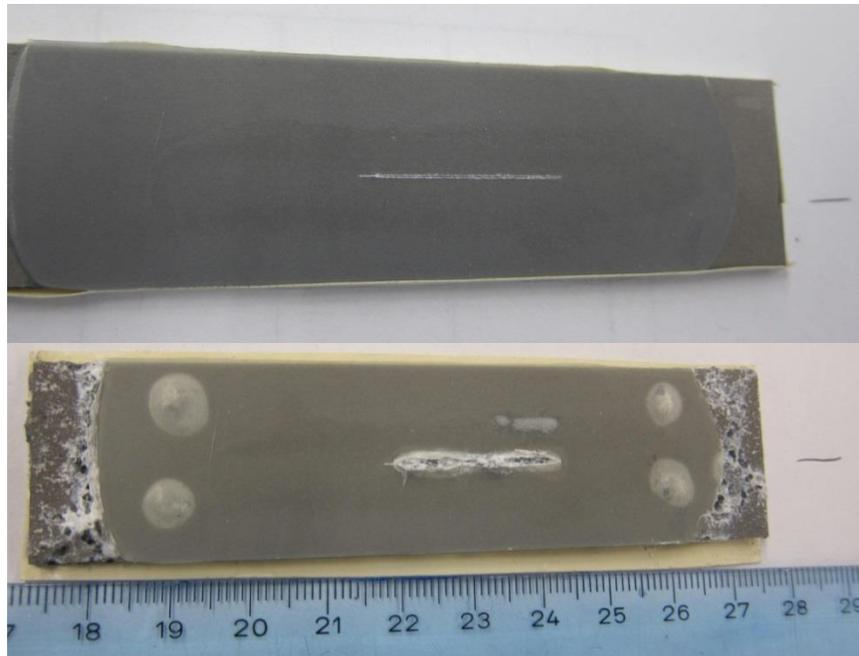
Figure 3-30: Open sandwich sample. DP460NS, Magnesium AZ31b, Gritblasting. (Before exposure [T], after exposure of 24 hours [B])
