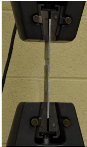
Figure 3-13: Lap shear sample located in the test jaws
