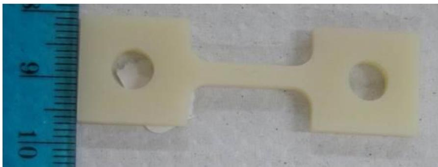
Figure 2-12: Bulk tensile sample geometry, micro-sized
