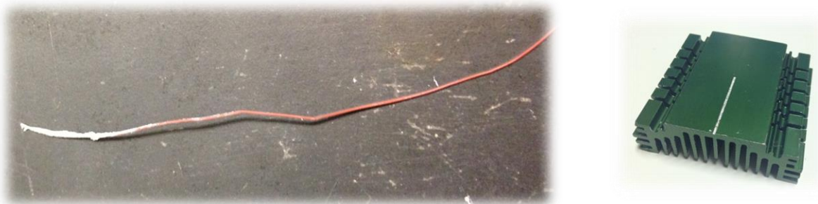
Figure 3.11: T-Type Thermocouple for Insertion into Single Channel on Heat Sink Bottom
