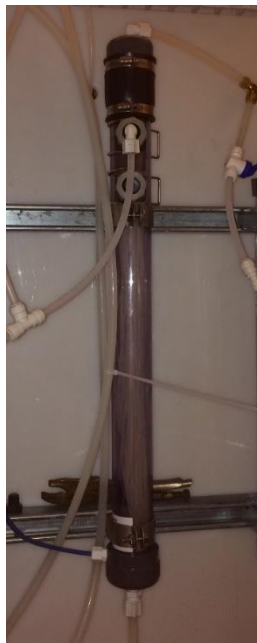
Figure 5-1 Zeeweed 1000 module (membrane fibers inside of housing)
