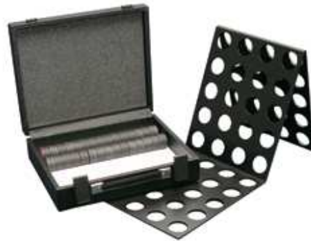
Figure 6: Minnesota Manual Dexterity Test (Lafayette Instrument, 1999) used for the hand and forearm dexterity task.
