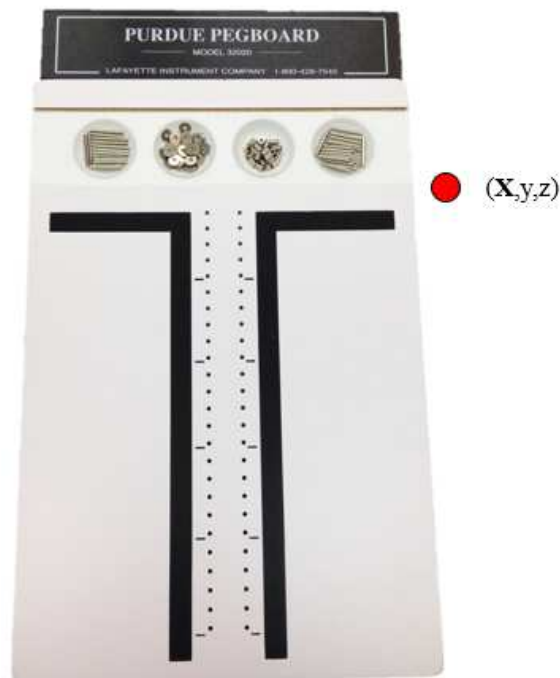
Figure 9: Diagram of equipment calibration for the fingertip dexterity task. A reflective marker (represented by the red dot) was placed at the base of the pin storage area and the position of the marker in the X direction was extracted, because movement is largely in the X direction for this task. Every time the hand markers passed the position of the marker, it signaled the start or end of a cycle.
