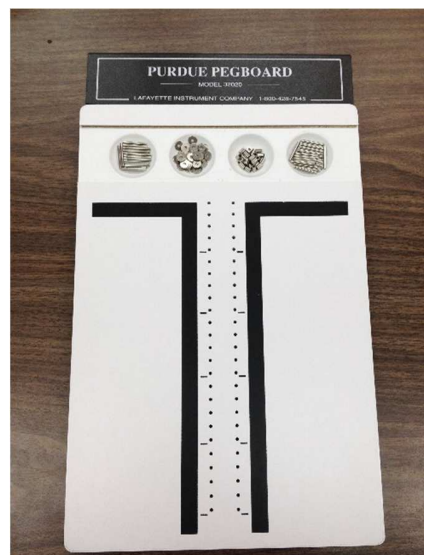
Figure 4: Overhead view of the Purdue Pegboard (Lafayette Instrument, 1999) used for the fingertip dexterity task.
