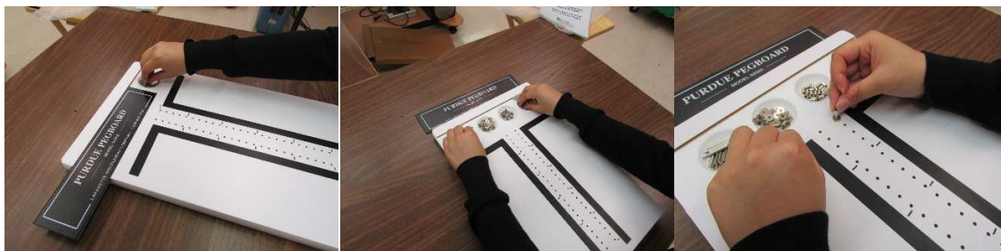
Figure 5: The Right Hand (left), Both Hands (middle), and Assembly (right) tasks of the Purdue Pegboard. The Left Hand task mirrors that of the Right Hand.
