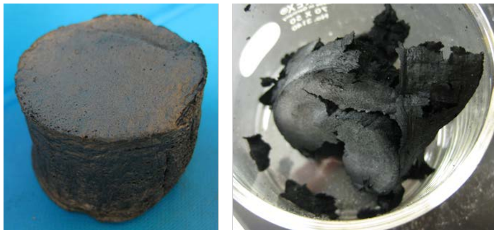
Figure 9. Photographic comparison of GO foam undergoing a slow and rapid thermal reduction
