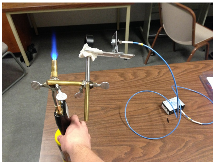
Figure 2.4: Bernzomatic Torch Optical Rig for Mark-1 Nebulizer Generation 1.
