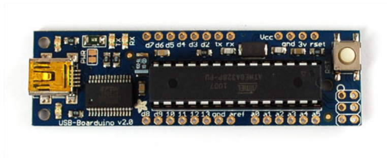
Figure 5.7: Populated BoArduino as used in the FAES system. [81] Digital pins d7→d2 are located in the top left pin header; digital pins d8→d13 are located in the bottom left pin header; the bottom right pin header is analog inputs; and the top right pin header is power.
