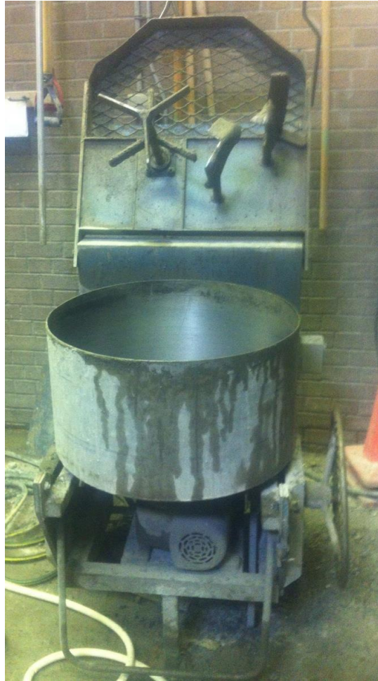
Figure 8.3: Rotary mixer for concrete mixing
