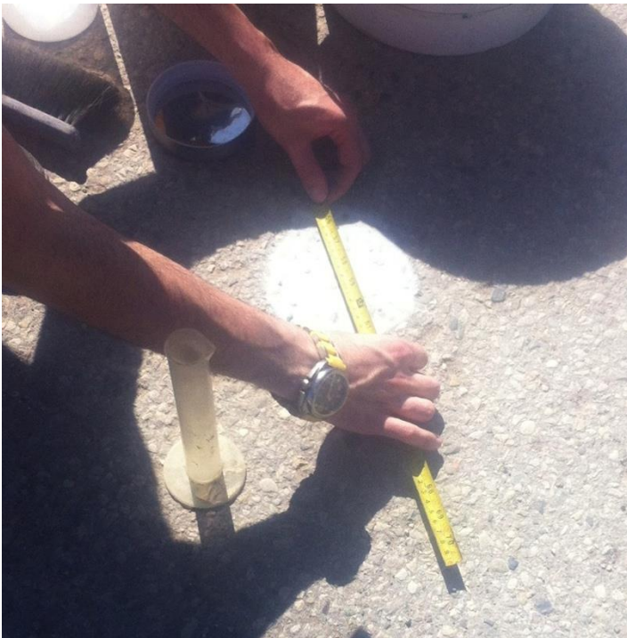
Figure 8.34: Sand patch test being conducted on asphalt road
