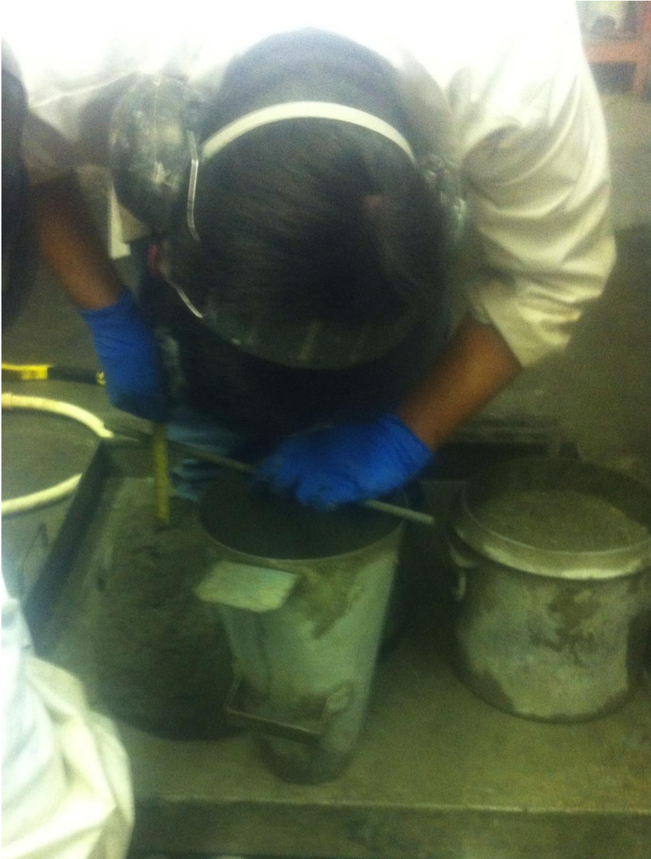
Figure 8.6: Slump test being performed on the concrete to ascertain workability
