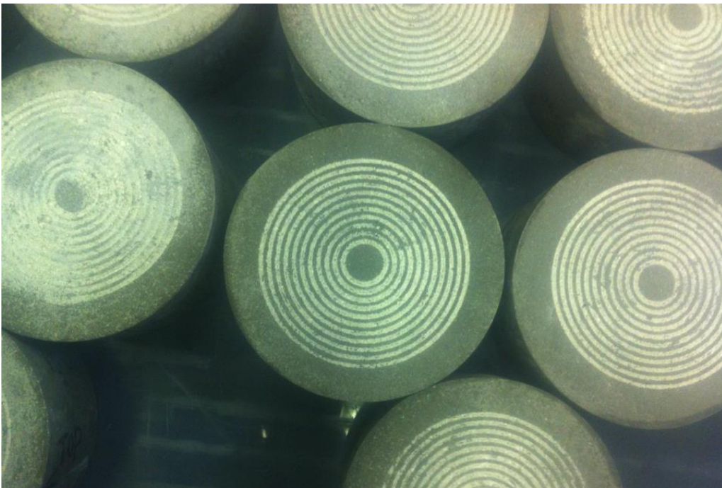
Figure 8.31: Concrete samples after the abrasion test (will be discarded after this test)
