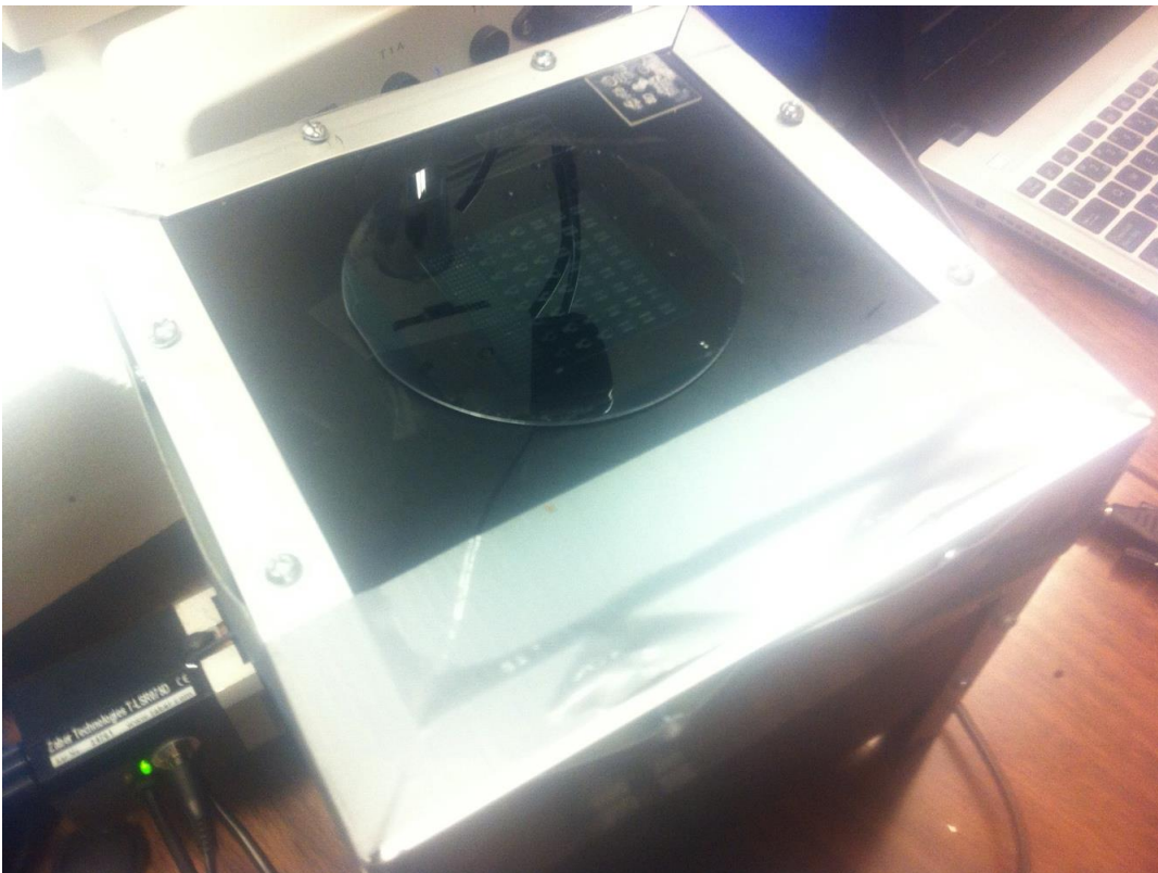
Figure 6.11: Playing fields for EMMA setup for ICRA competition 2014. A large number of fields are etched on a single silicon wafer.
