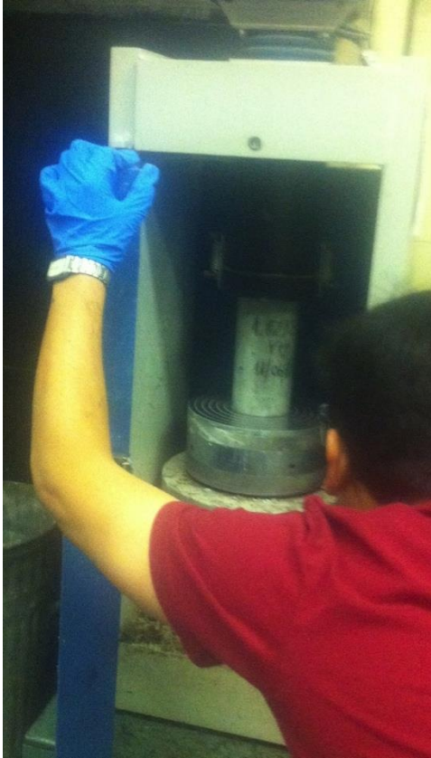
Figure 8.17: Ensuring that the compression head of the machine merely touches the top of the surface before beginning the test
