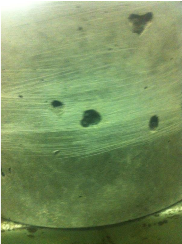
Figure 8.14: Air voids formed in the concrete sample (found after demolding)
