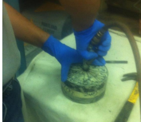
Figure 8.11: Air being passed from the bottom for easy demolding
