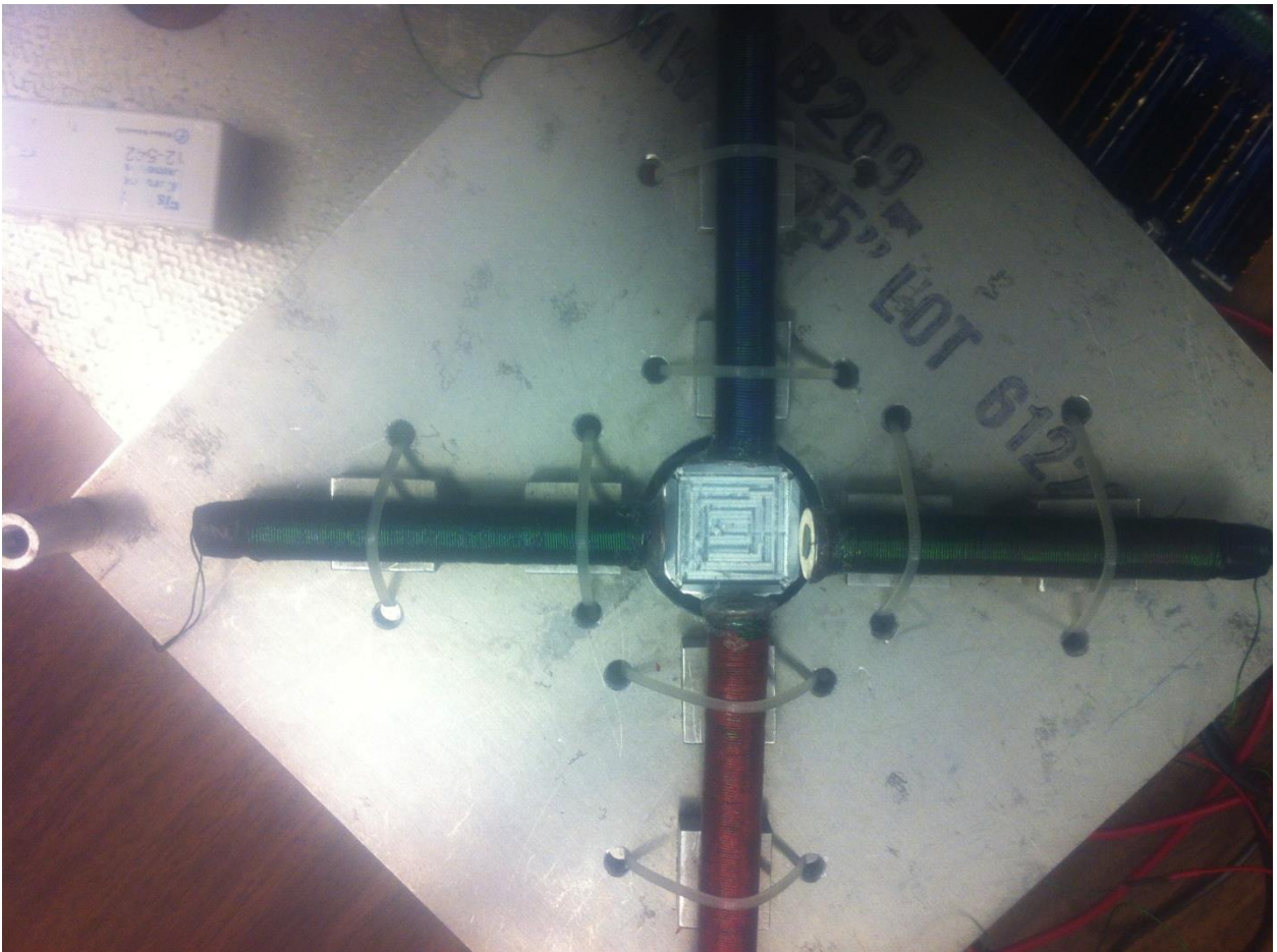
Figure 6.19: SAM setup in this form is provided to save the robotic playing field from dust. The figure shows the playing fields surrounded by four electromagnets (long metal rods with red and green wires).
