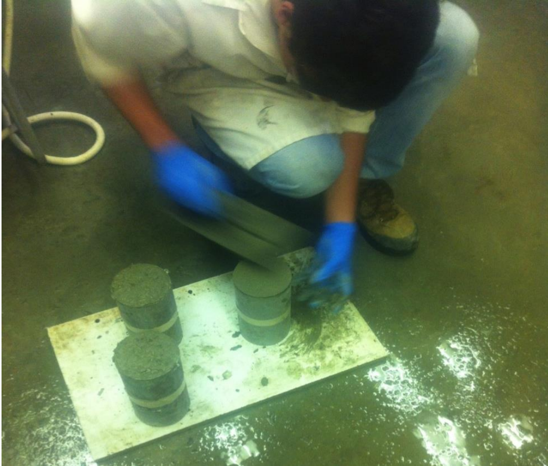
Figure 8.9: Molds being given a plane surface finish
