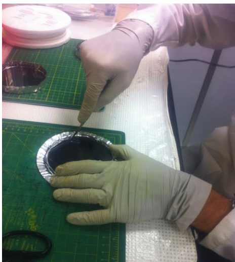
Figure 4.11: Cutting the PDMS from the mold. The knife is used at the edges to ensure that the mold is not destroyed. The freed PDMS will subsequently be sliced into smaller pieces.
