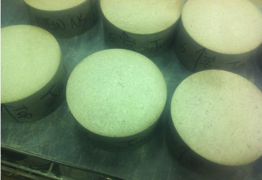
Figure 8.13: Molded concrete samples with flat surface
