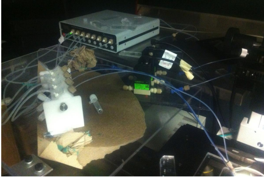
Figure 4.13: Setup for testing. Pressure pump is connected to the inlet and outlet of the microtubules. The tubes are provided connecting the pressure pump and LOC device in a closed flow circuit. The computer is connected to the microscope for a closed loop for information and data collection.
