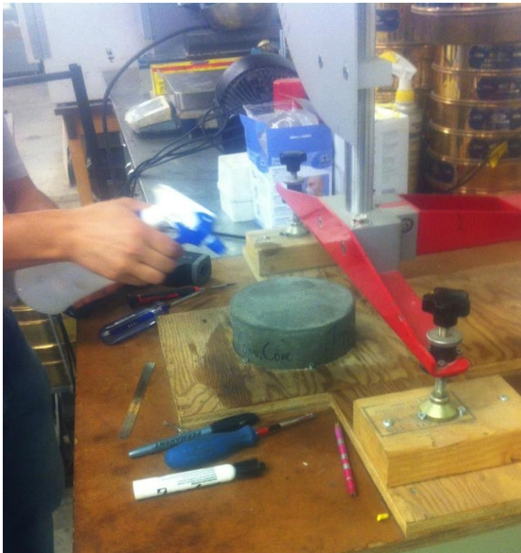
Figure 8.23: Nanoconcrete sample being setup in the British Pendulum Test
