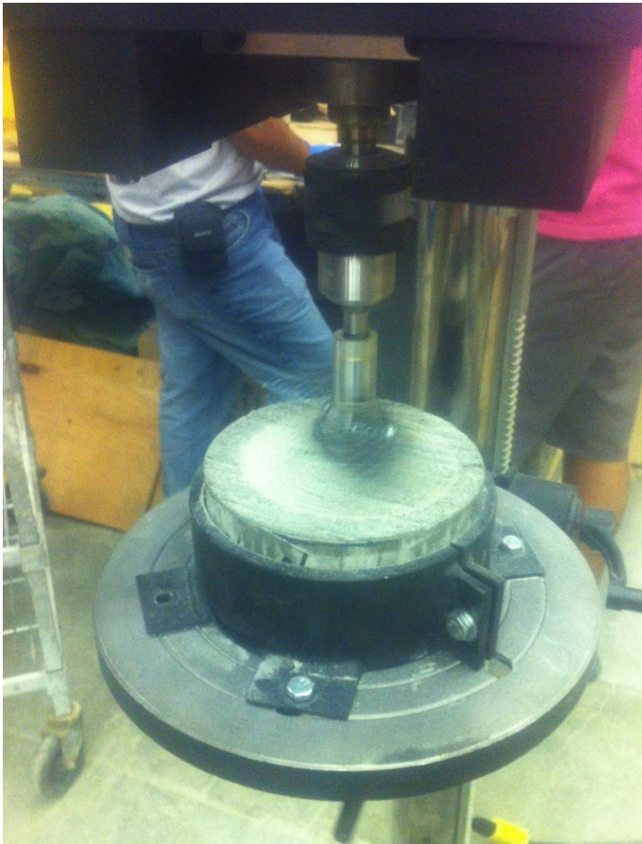
Figure 8.29: Abrasion test in progress
