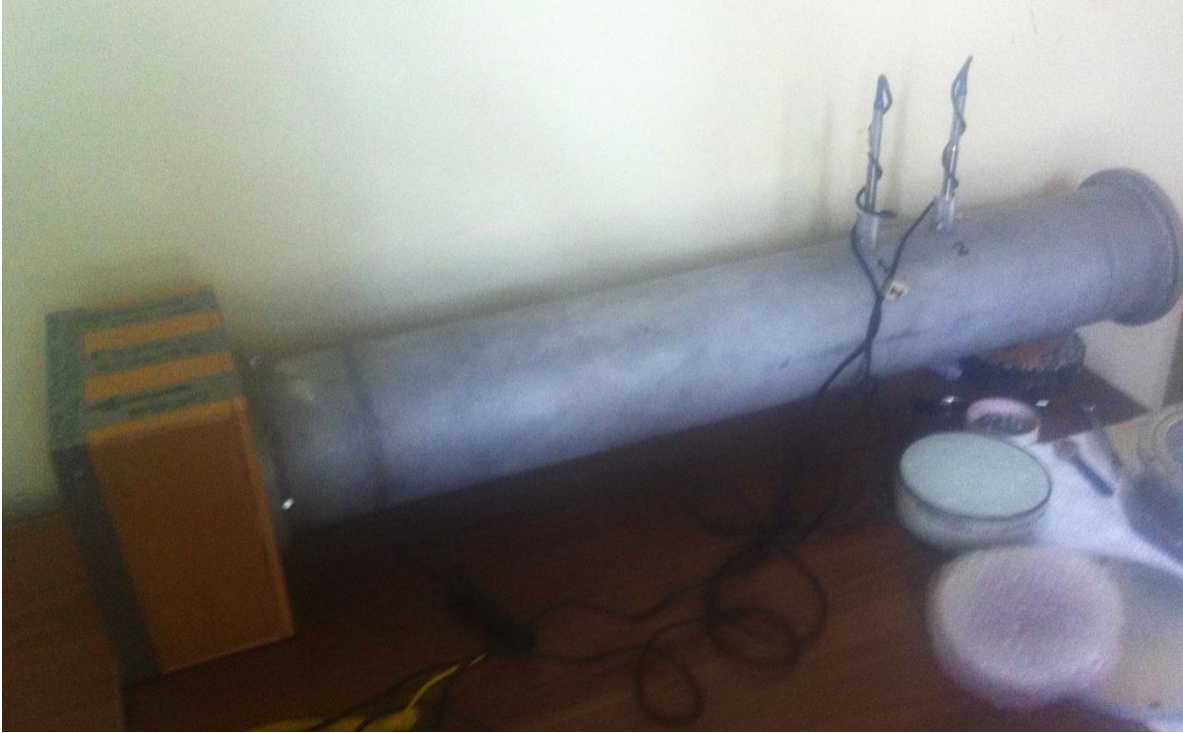
Figure 8.20: Sound absorption test equipment
