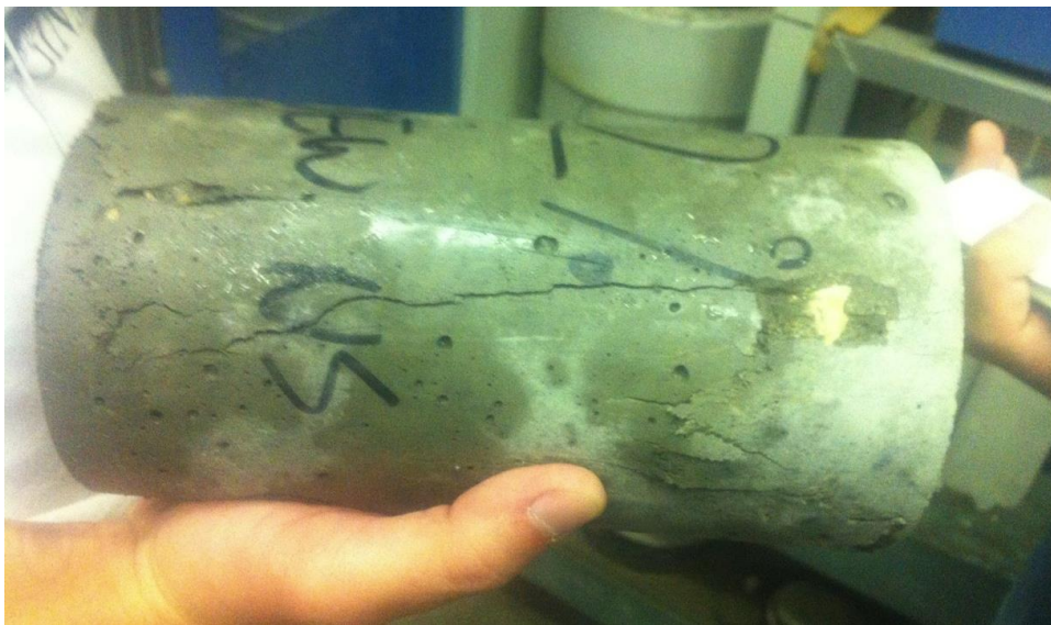
Figure 8.19: Cracked sample, after the compression test
