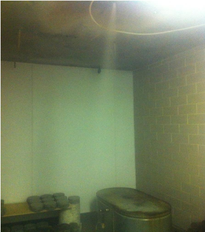
Figure 8.15: Humidity chamber for curing. Notice the thin jet of water from the top of the room to provide constant humidity
