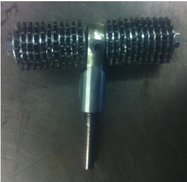
Figure 8.28: Rotatory head used for the abrasion test
