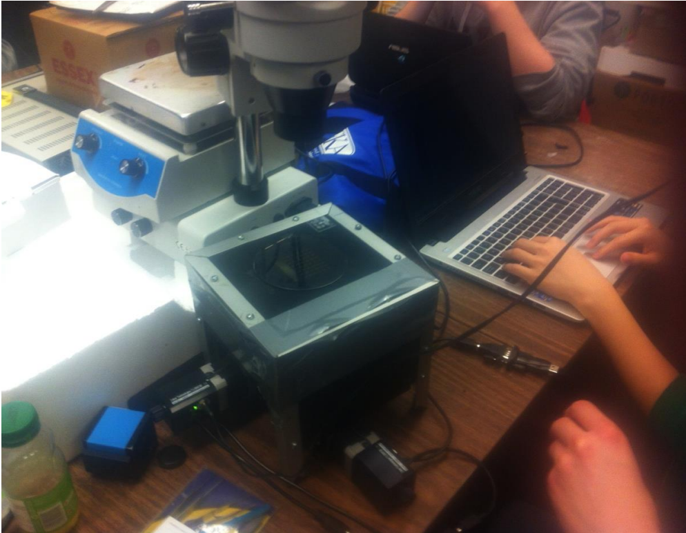
Figure 6.12: EMMA setup being prepared for the completion for 2014. The actuator is below the robotic playing field. The microscope is above the playing field. Both the microscope and the actuators are connected to form a closed loop setup.
