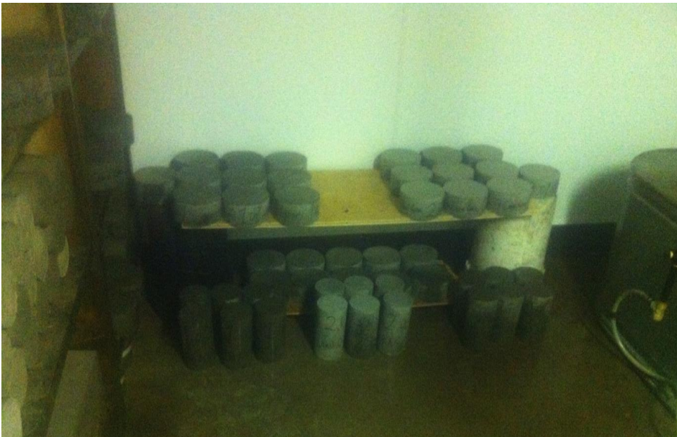
Figure 8.16: Samples placed in the humidity chamber for curing
