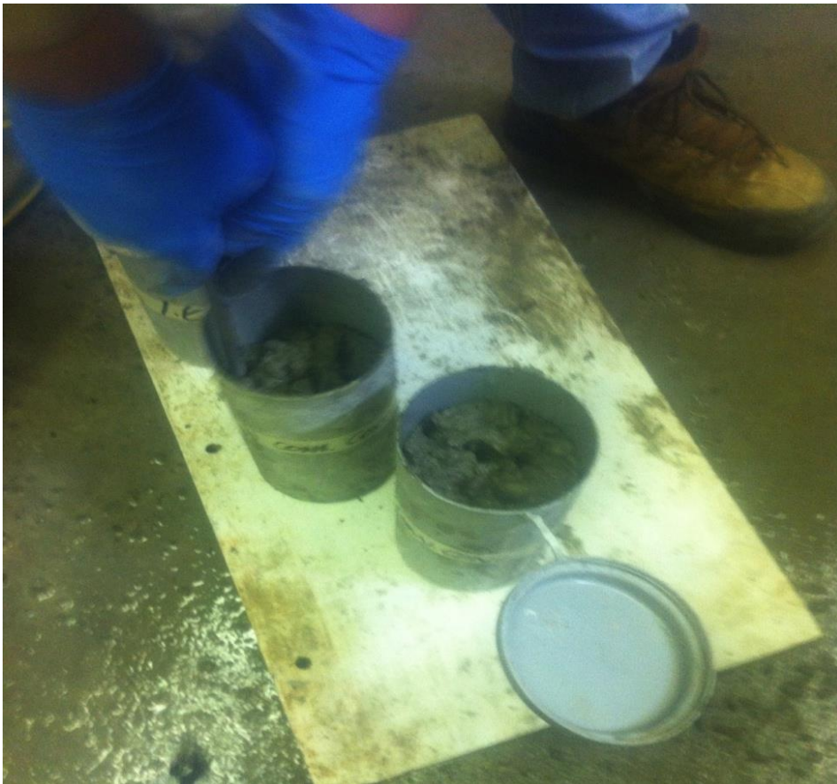
Figure 8.8: Molds being poked by a rod to enable the settling of concrete
