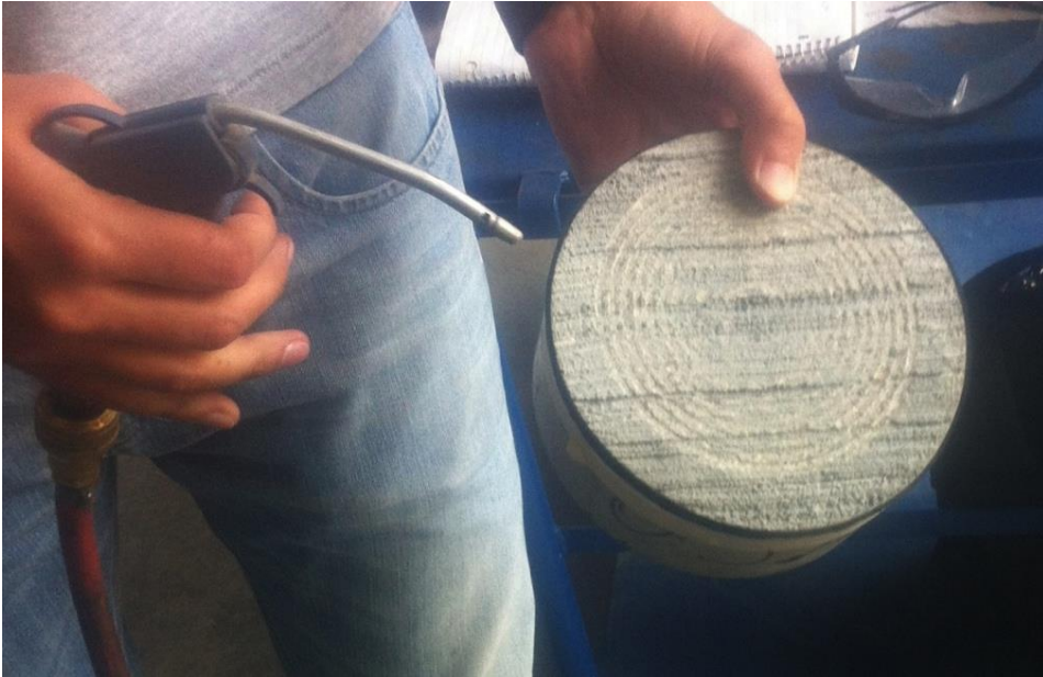
Figure 8.30: Cleaning the mold with a blast of air to get rid of the dust after the abrasion test
