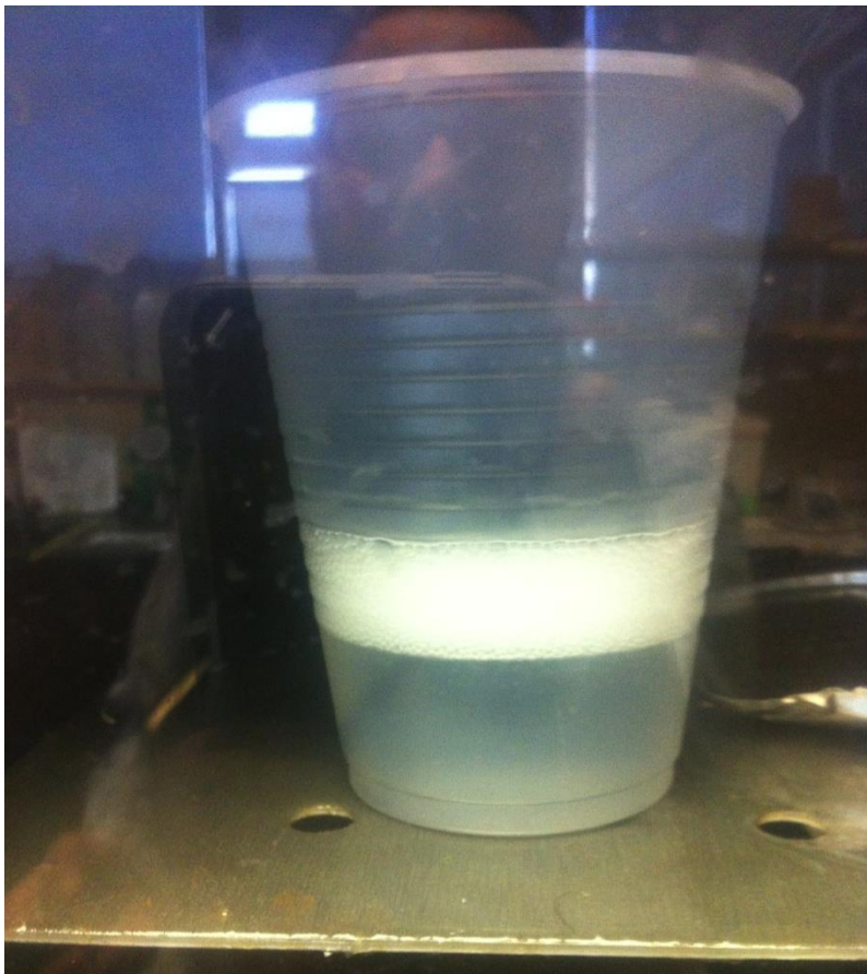
Figure 4.8: The white froth is air bubbles. For removing the air bubbles, it is placed in the degassing chamber
