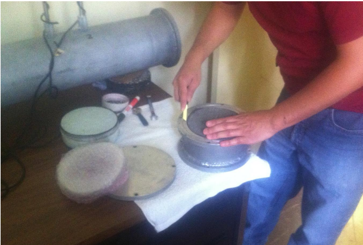
Figure 8.21: Fitting the mold into one end of the equipment
