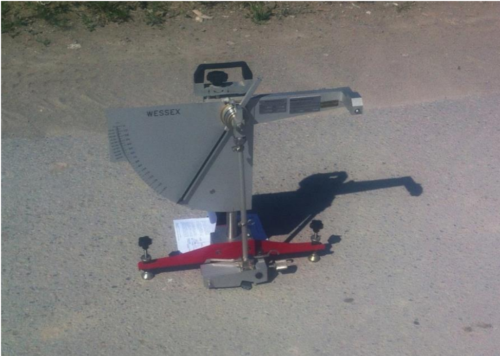
Figure 8.33: British Pendulum Test to be conducted on the asphalt and concrete roads
