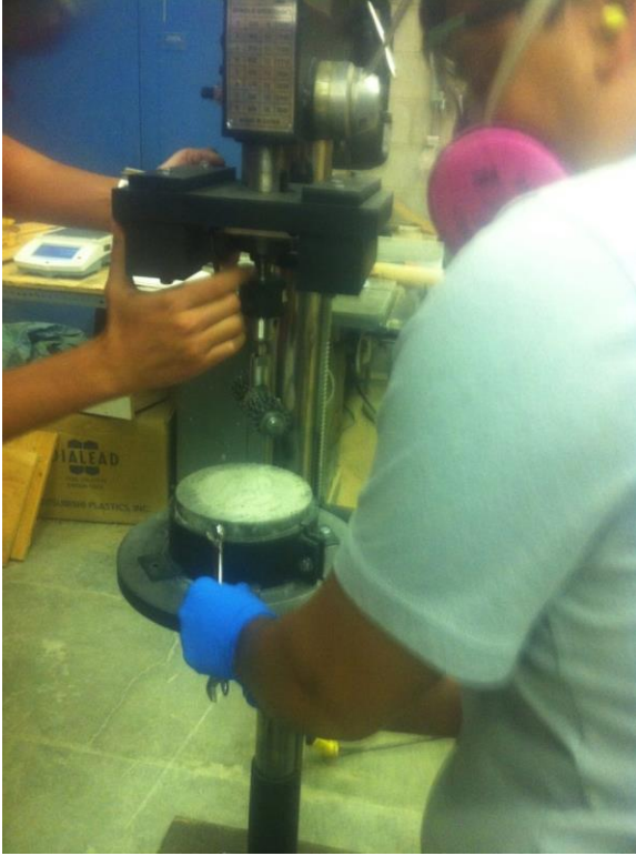
Figure 8.27: Setting up the abrasion test equipment
