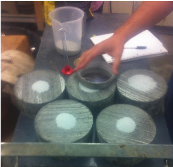
Figure 8.25: Spreading the sand in a circular form
