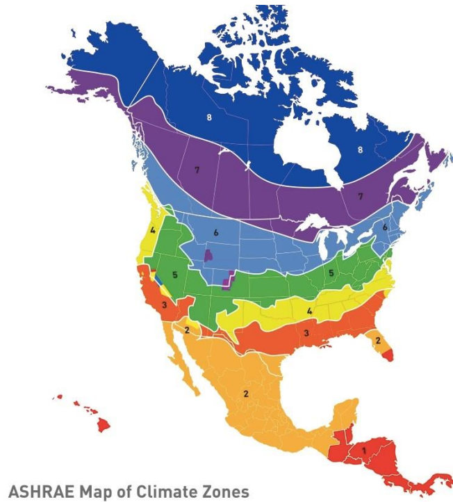
Figure 2-10 North America Region climate zone by ASHRAE Standard 90.1 (reproduced from ATLAS Building Forward (ATLAS 2014))
