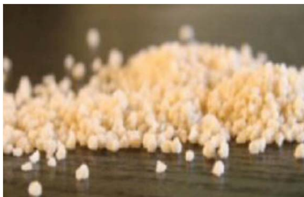
Figure 8. EcoSphere TM starch nanoparticles agglomerate produced from extruder. Image is adapted from ref. 72
