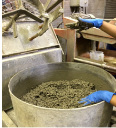
Figure 4-1 Mixing Materials in the Mixer
