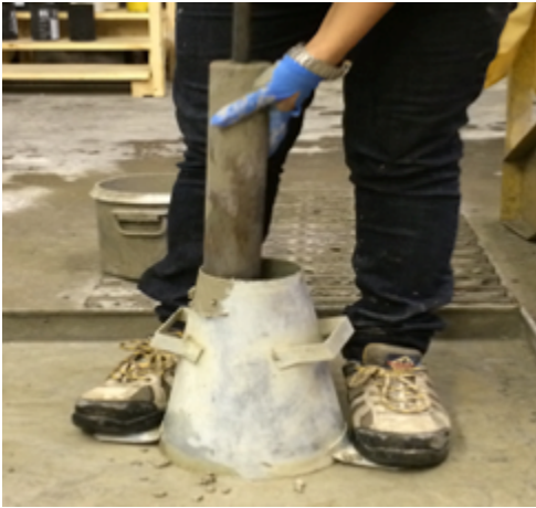
Figure 4-2 Hammering For Slump Test
