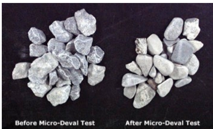
Figure 2-4 Aggregate particles before and after Micro-Deval test (Pavement Interactive, 2011)
