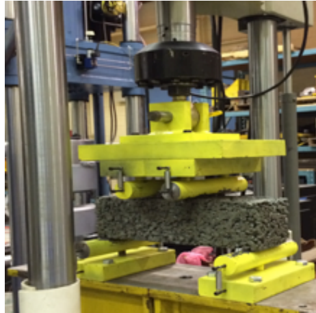
Figure 4-8 Flexural Strength Testing
