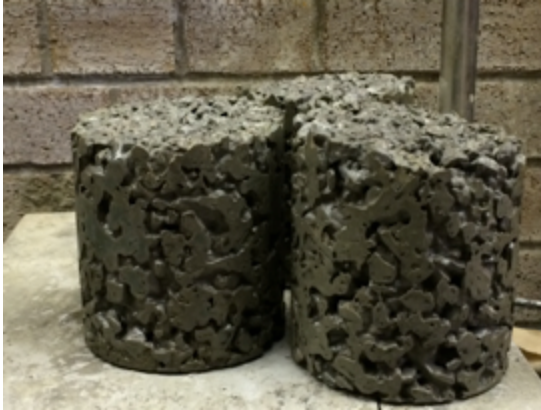
Figure 4-12 Sample set Before and Figure 4-13 Sample set After LA Abrasion Test
