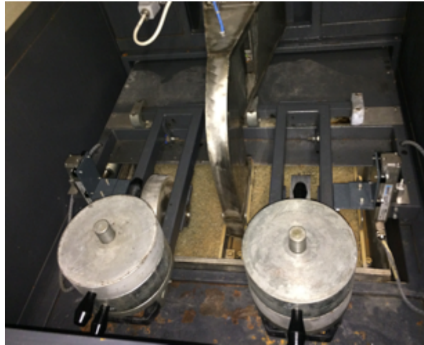
Figure 4-14 Hamburg Wheel Rutting Testing
