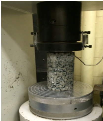
Figure 4-7 Compressive Strength Testing
