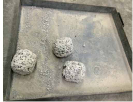
Figure 4-12 Sample set Before and Figure 4-13 Sample set After LA Abrasion Test
