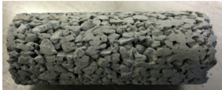
Figure 2-1 Pervious Concrete Core
