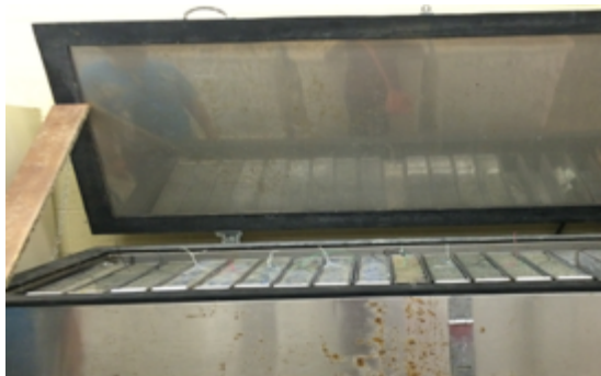
Figure 4-15 ASTM C666 Procedure (A)
