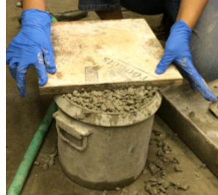
Figure 4-5 Striking off excess material
