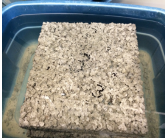
Figure 4-18 Scaling Samples submerged in the salt solution
