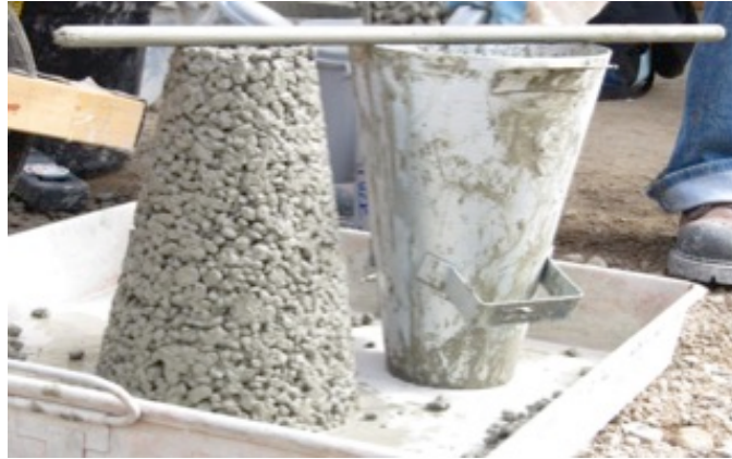
Figure 2-6 Pervious concrete slump testing (Henderson, 2012)
