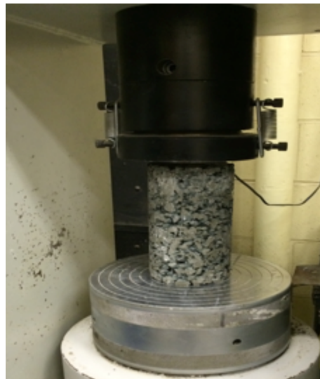
Figure 2-7 Pervious concrete sample undergoing compressive strength testing
