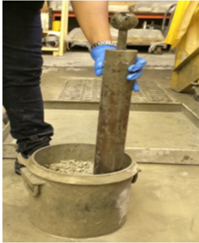
Figure 4-4 Compacting with Proctor Hammer
