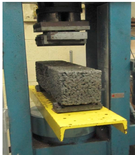
Figure 2-8 Pervious concrete sample undergoing flexural strength testing (Henderson, 2012)
