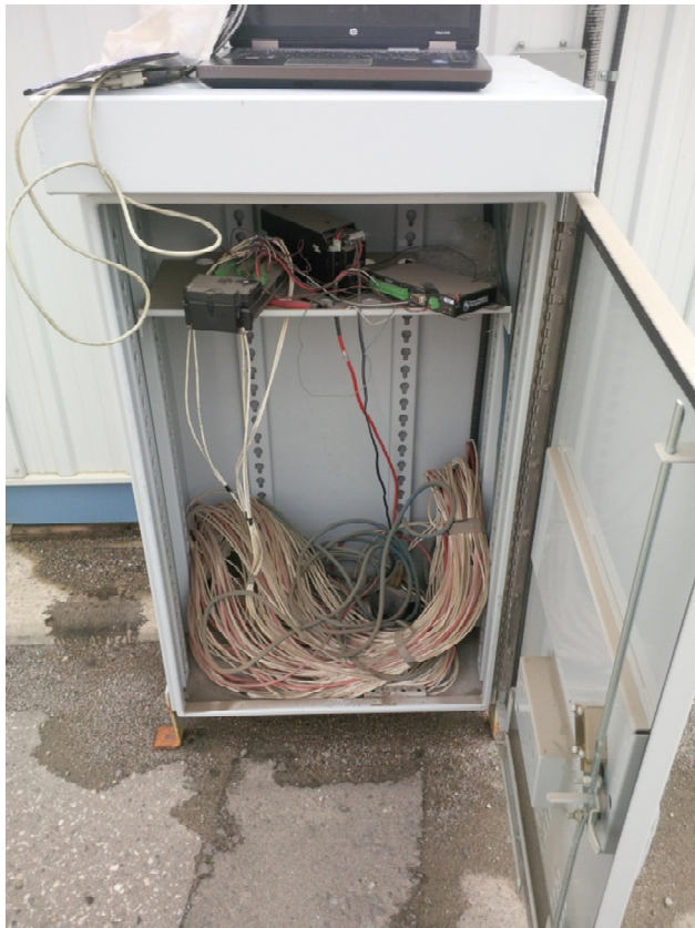
Figure 24 - CR-1000 Data Logger and Field Setup
