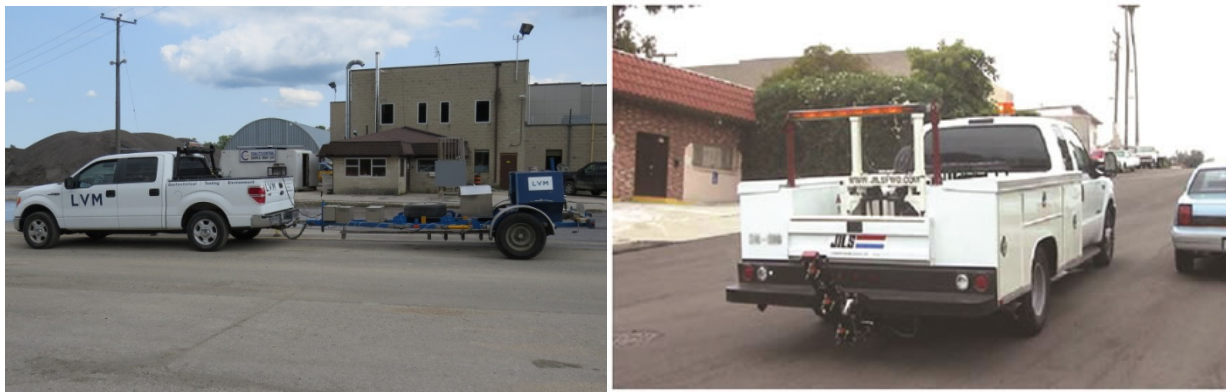
Figure 7 - Truck and Trailer Mounted FWD Devices [Duclos, 2014; FHWA, 2011]
