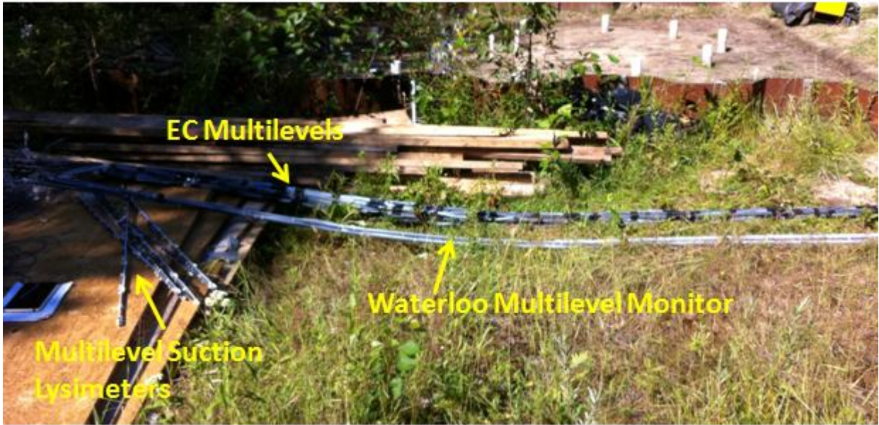
Figure 2.7: Different types of new monitoring wells for Borden sulfate land application.
