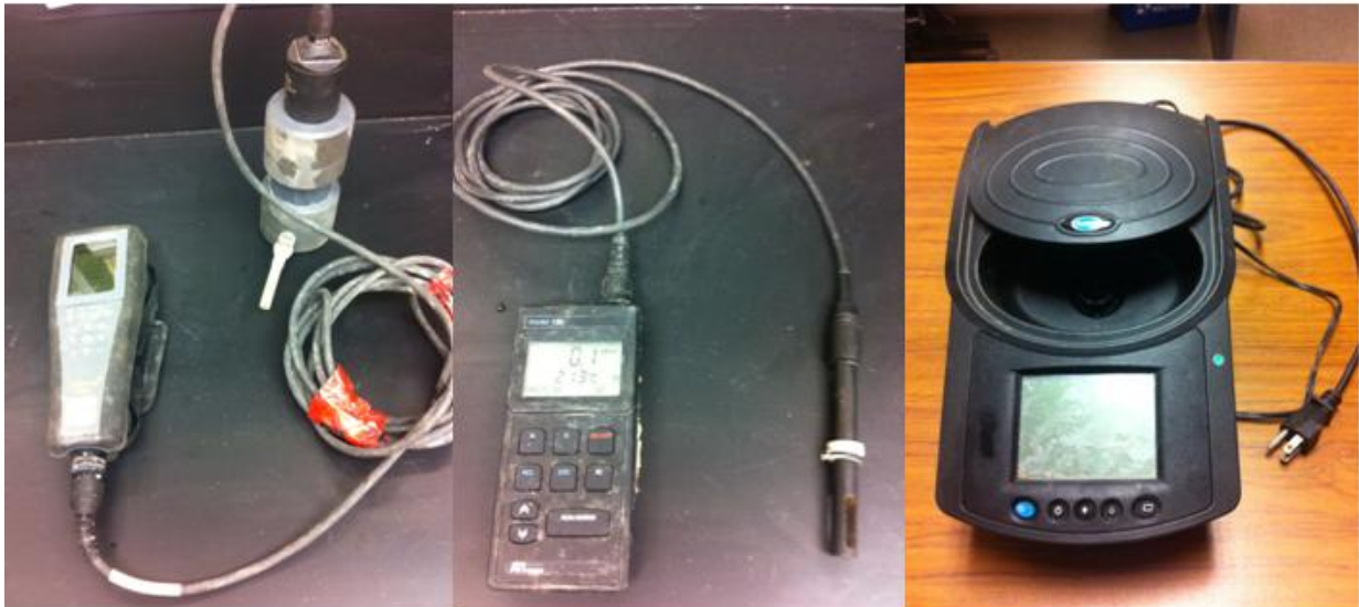
YSI Professional Plus meter with flow-through cell
