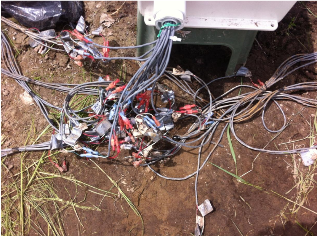
Figure 3.3: Connection between data logger and probe lead extensions at field.
