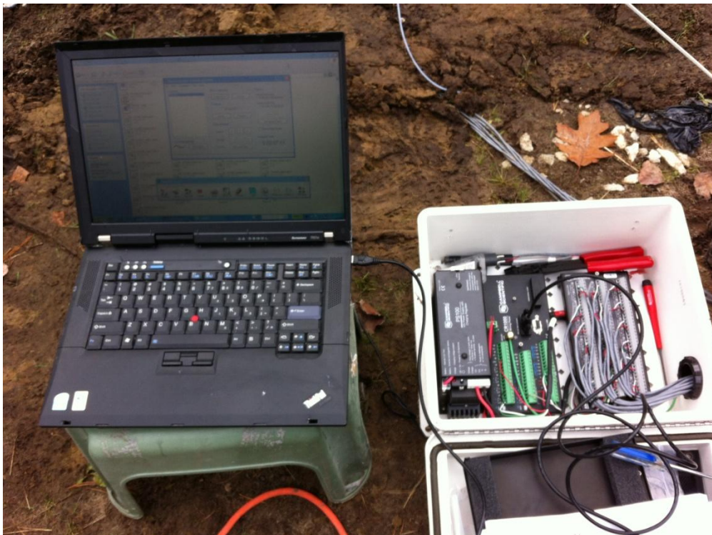
Figure 2.12: Data logger field data viewing. Field laptop and data logger connected by USB/RS 232 cable.
