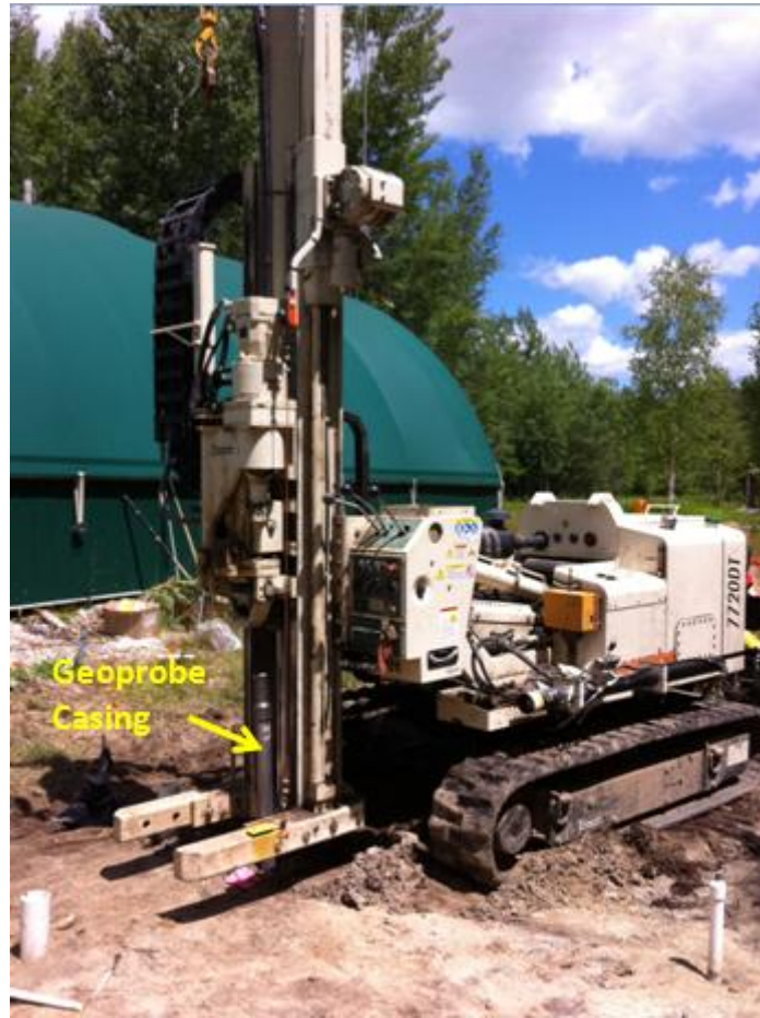
Figure 3.1: Geoprobe® 7720DT at Borden field. Another casing would be added to the top of the previous one as the pushing proceeded.
