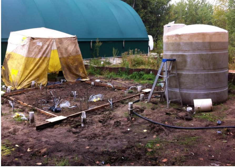
Figure 4.1: The pond created by planks and bermed sand. Prepared sulfate water stored in the tank to the right of the pond area.
