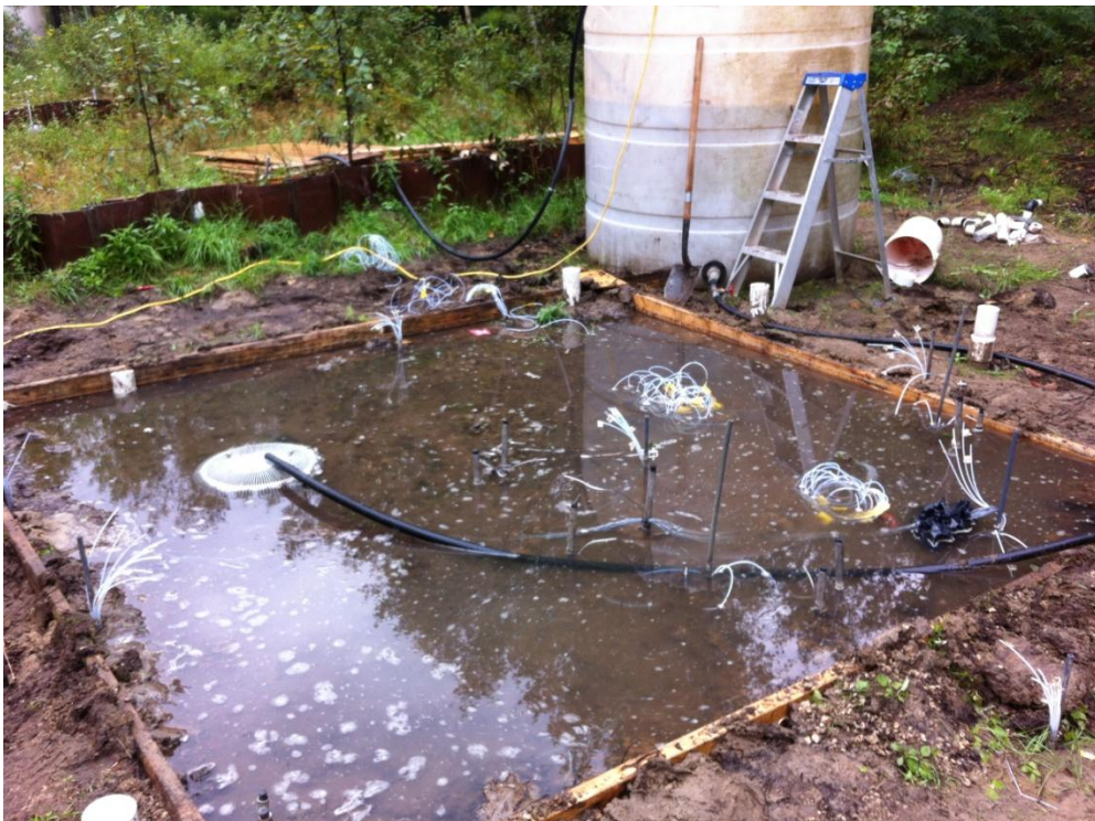
Figure 4.2: Bermed pond at constant water level during the first application.
