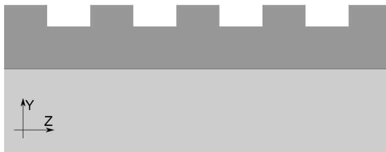
Figure 6: Side view of grating coupler Mode propagates in z direction
