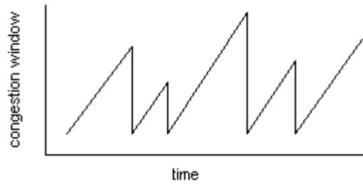
**Figure 9:** Saw-tooth profile of TCP congestion window.
