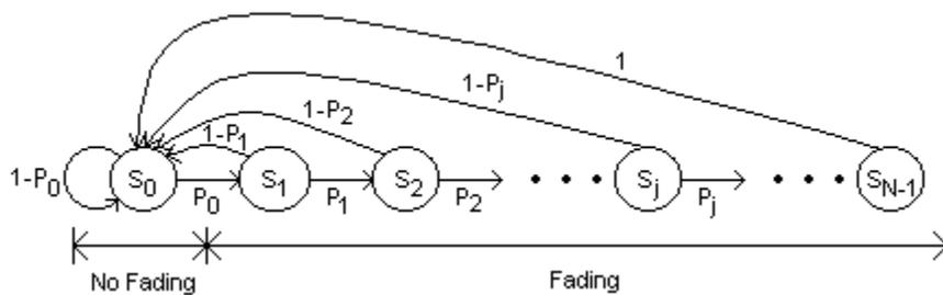
**Figure 25:** N-state Markov channel model.
