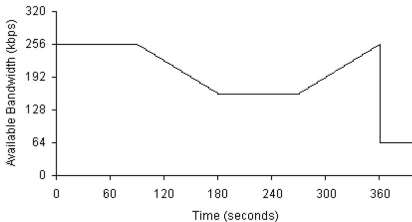
**Figure 23:** Wired network congestion profile for simulations.
