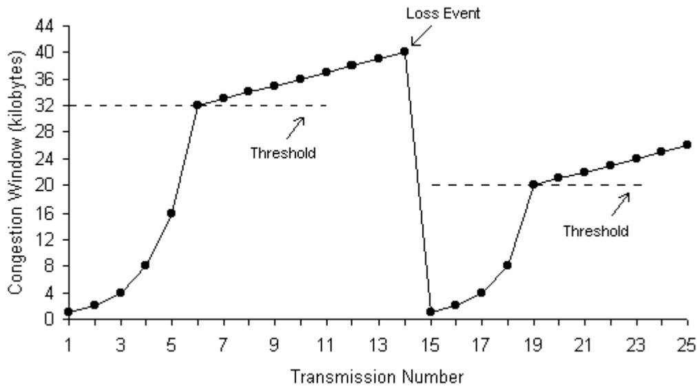
**Figure 6:** Example of TCP congestion control algorithm.
