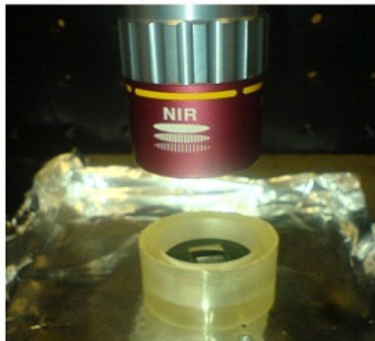
Figure 4-1 Sample held in liquid media with 4mm liquid on the surface
