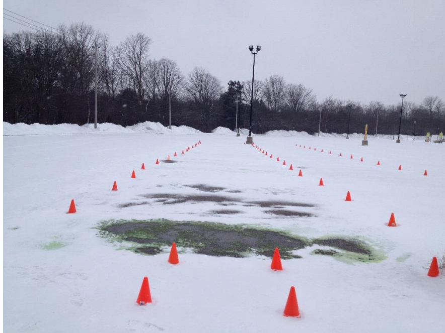
b) Set-up for Testing Organic Salts (e.g., Green salts)
