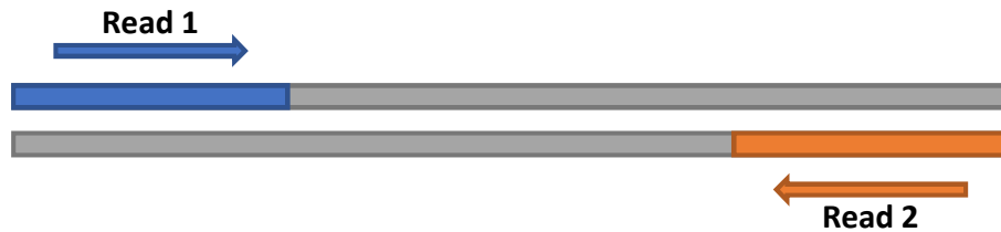
Figure 1.1: An example of paired-end sequencing. The pairs of reads are sequenced from the same fragment with Read 1 sequenced in the forward direction and Read 2 sequenced in the reverse direction.
