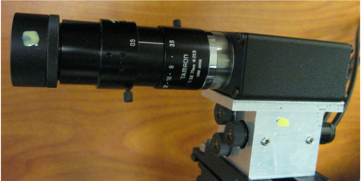
Figure 5.2: Photo of the camera and beacon laser system used for tracking. Three lasers are used for extra power and for redundancy should one fail during the experiment. Both the transmitter and receiver are equipped with this camera and laser system, allowing each camera to track the other's lasers. The camera has a field of view of 4.73^\circ in one axis (1024 pixels) and 5.91^\circ in the other axis (1280 pixels), corresponding to an accuracy of 0.0046^\circ/\text{pixels} .
