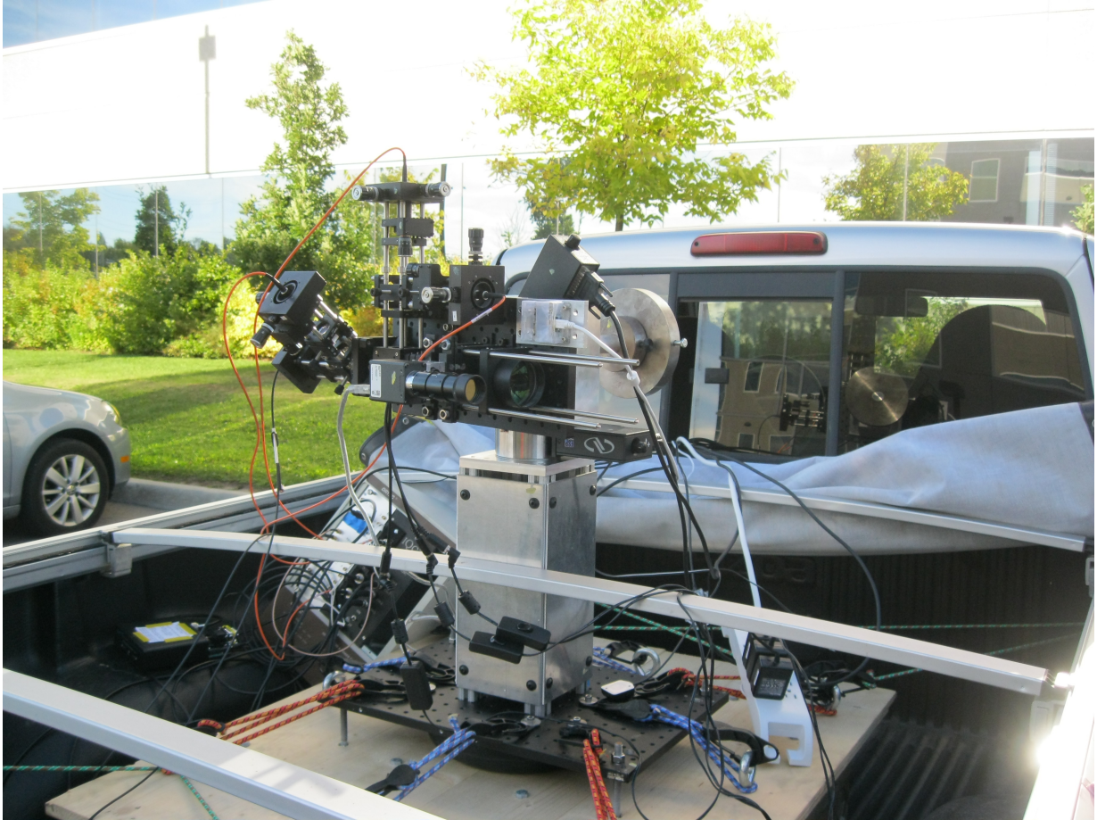
Figure 5.6: Photo of the moving receiver platform. The receiver system is mounted on a wooden platform using bungee cords and an inner tube which act as a suspension system to reduce vibrations. The wooden platform is attached to the truck using bungee cords at all four corners, acting as an additional suspension system in the horizontal plane (the weight of the platform, \approx 50 kg, and its low center of mass prevent any significant vertical movement relative to the truck bed).
