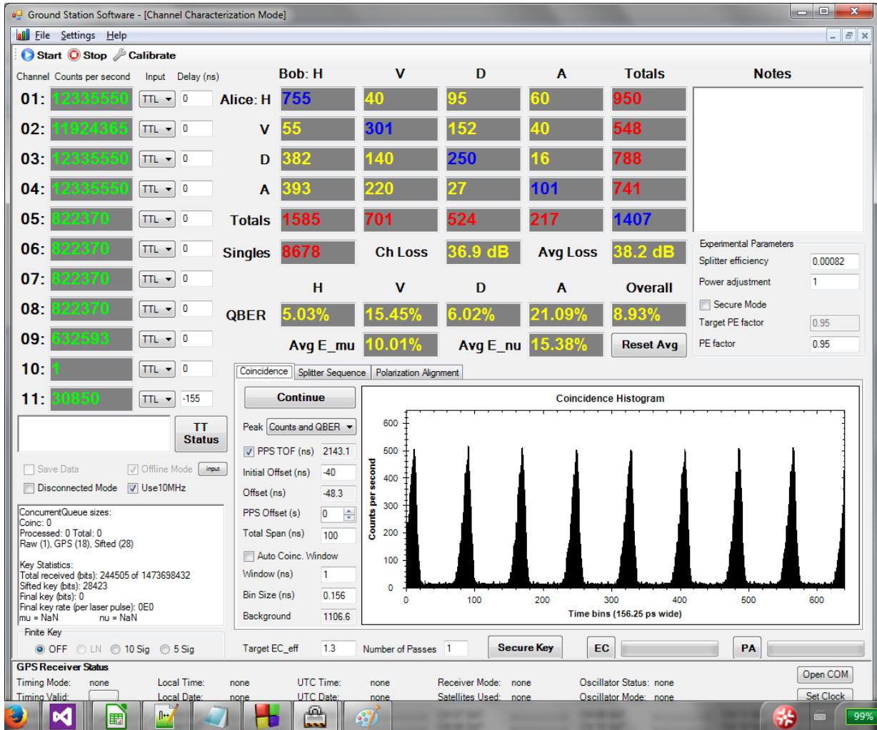
Figure 5.26: Snapshot of the user interface showing quantum signal peaks during 1 s of the 20 km/h test. The background level can also be seen at the base of the peaks. Once again the width of the signal peak is determined by the combined contributions of the laser pulse width ( \approx 50 fs, negligible), the drift in the repetition rate of the pulsed laser (typically a few 100s of ps), the detector timing jitter ( \approx 600 ps, includes detector electronics), the timing accuracy of the time-tagger (156.25 ps) and the delay of the four detectors compared to each other (typically aligned within 100–200 ps).
