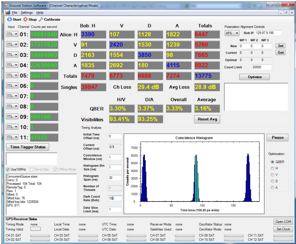
Figure 3.11: User interface at Alice showing the histogram-based optimizing coincidence search. The light blue area shows the counts captured with the optimal delay for the current second. This optimal is determined by identifying the signal peaks by finding the maximum count rates in each laser period, and then moving the delay across the peaks and optimizing the QBER. The width of the capture counts (light blue area) is determined by the coincidence window.
