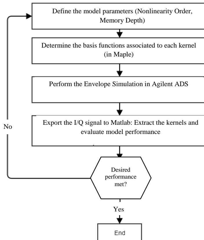
**Figure 3.6- Extracting Volterra DIDO Model**
