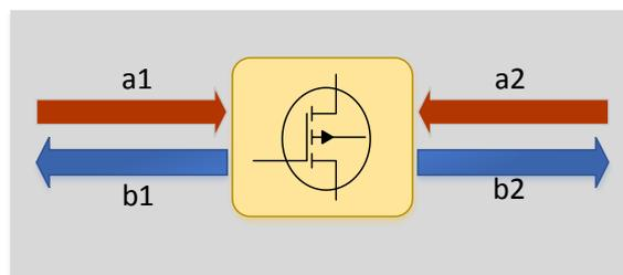
Figure 2.1 - Two-Port Device Representation
