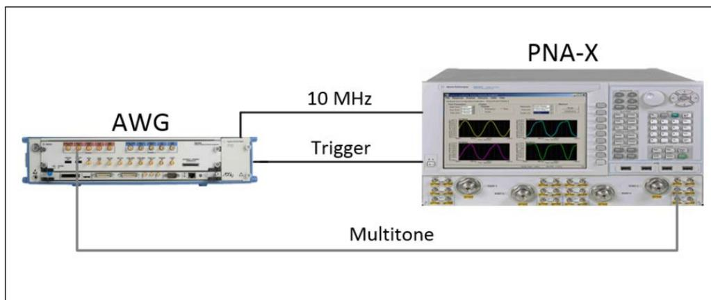
**Figure 4.5 - IF Calibration Setup**
