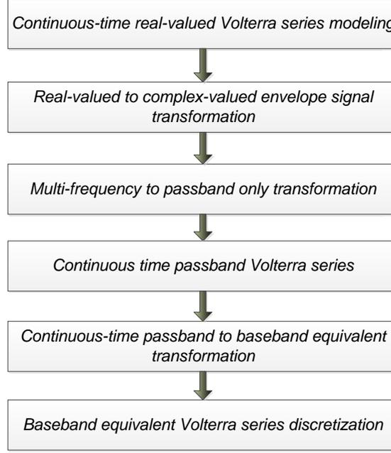
**Figure 3.1 - Baseband Equivalent Modeling Approach [26]**
