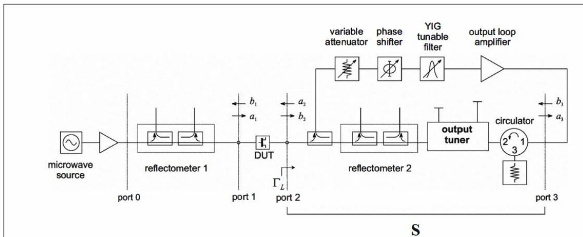
Figure 2.11 - Example of a Hybrid Load-pull [6]
