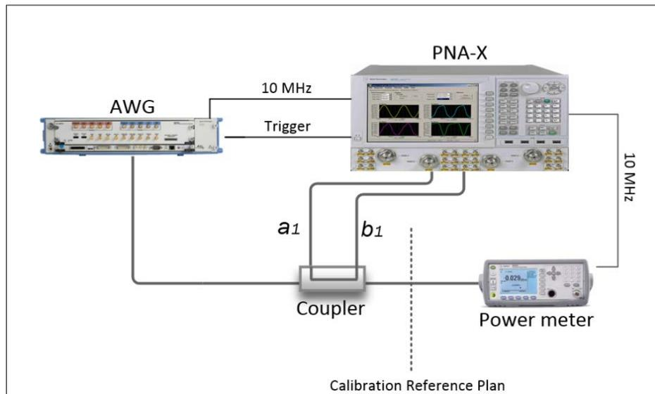
**Figure 4.10 – Absolute Power Calibration**
