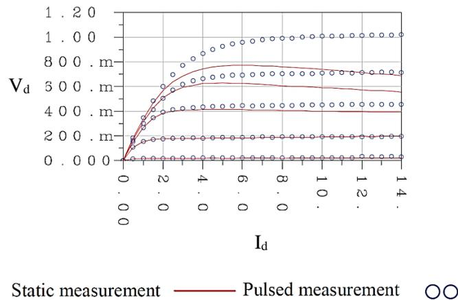
Figure 2.4 - Static IV vs. Pulsed IV measurement for a LDMOS Transistor [3]
