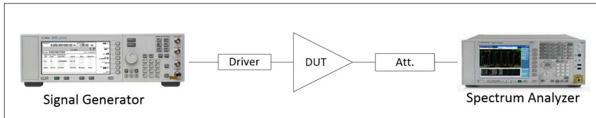
**Figure 2.2 - Measurement Setup for Matched Nonlinear Devices**
