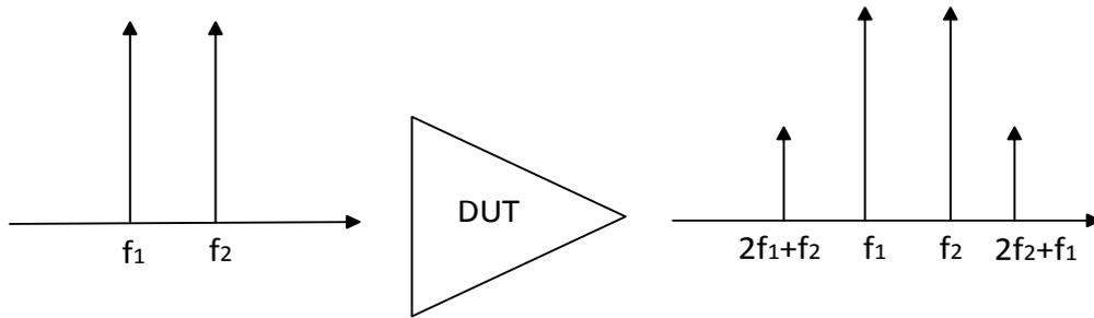
**Figure 2.5 - DUT 3<sup>rd</sup> Order Intermodulation**
