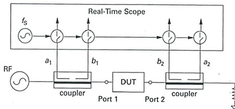
**Figure 2.6 – High-speed Scope Based Characterization Setup [1]**
