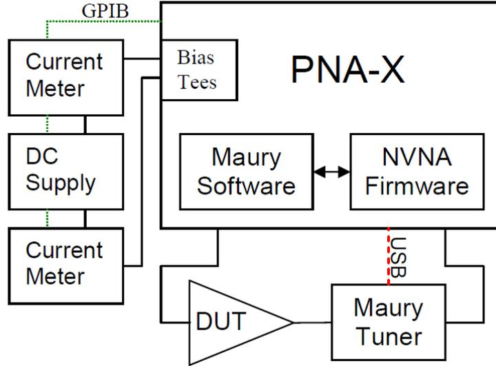
**Figure 2.15 - Measurement Setup for Load-dependent X-parameters [15]**
