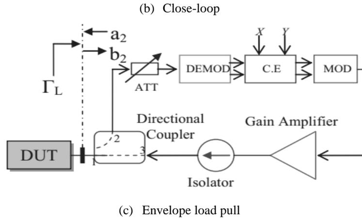
**Figure 2.10 - Active load Pull Configurations: (a) Open-loop, (b) Close-loop, (c) Envelope load pull [5]**
