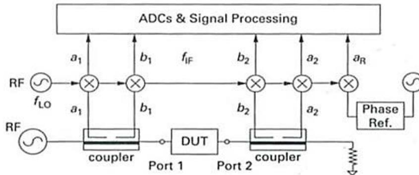
Figure 2.8 – NVNA Based Characterization Setup [1]
