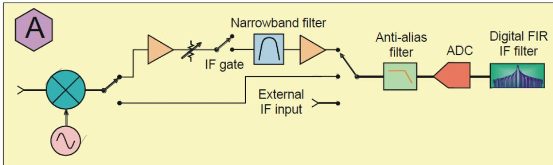
Figure 4.3 - Agilent PNA-X Receiver Block Diagram
