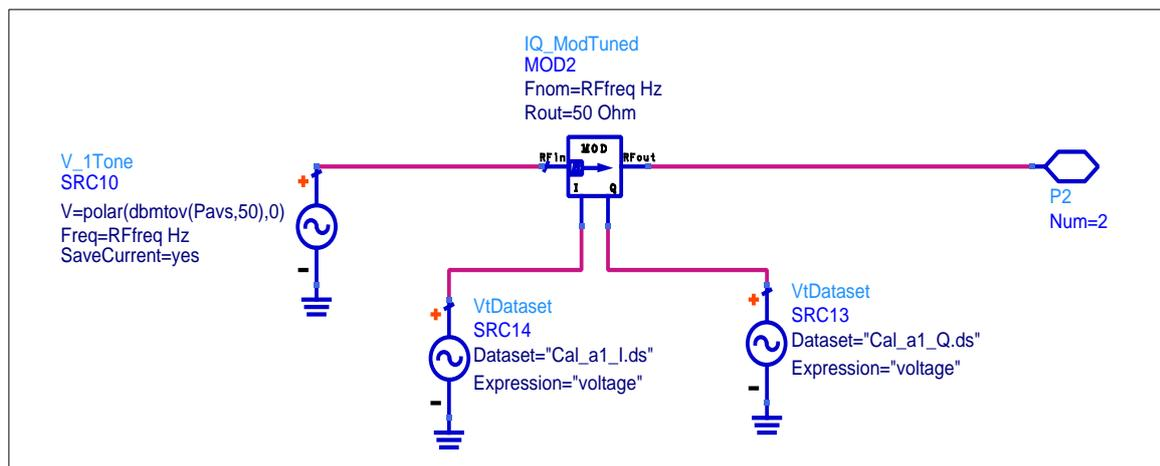
**Figure 3.4 - Modulated Signal Generation**
