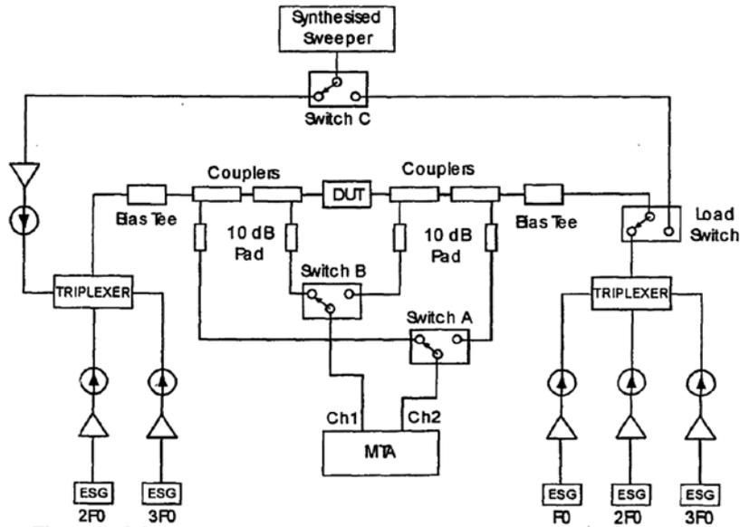
Figure 2.16 - Two-port Time Domain Measurement System [21]
