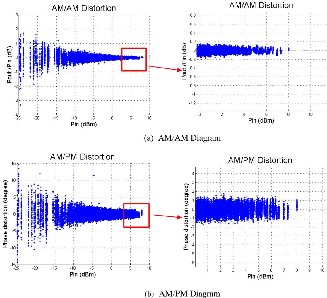
Figure 4.7 Receiver Characteristics (a) AM/AM Diagram (b) AM/PM Diagram
