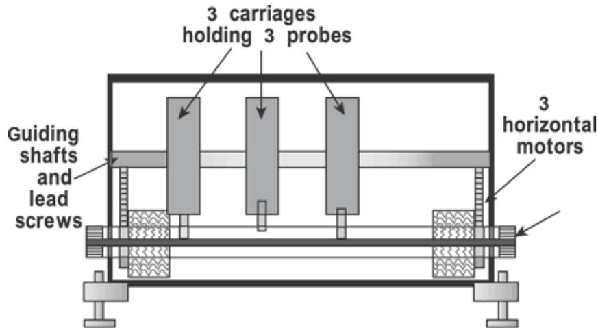
Figure 2.9 - Passive Tuner Diagram [4]
