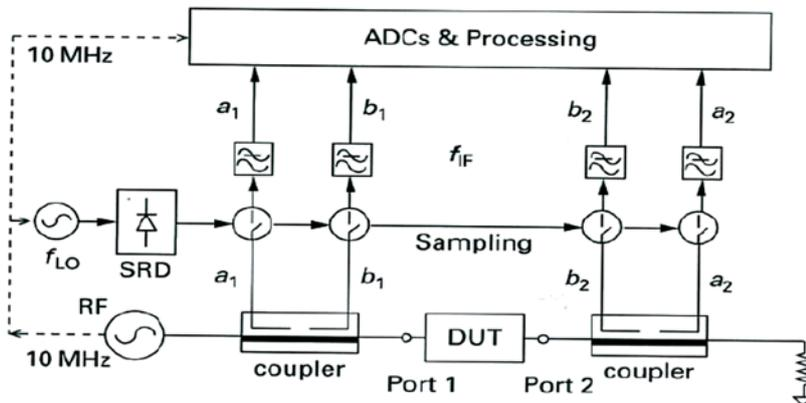
Figure 2.7– LSNA Based Characterization Setup [1]
