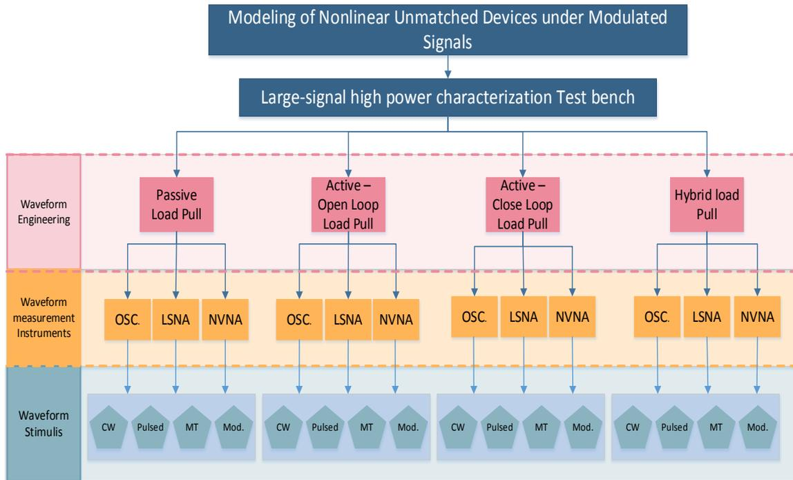
Figure 2.12 – Nonlinear Characterization Setup Structure Breakdown
