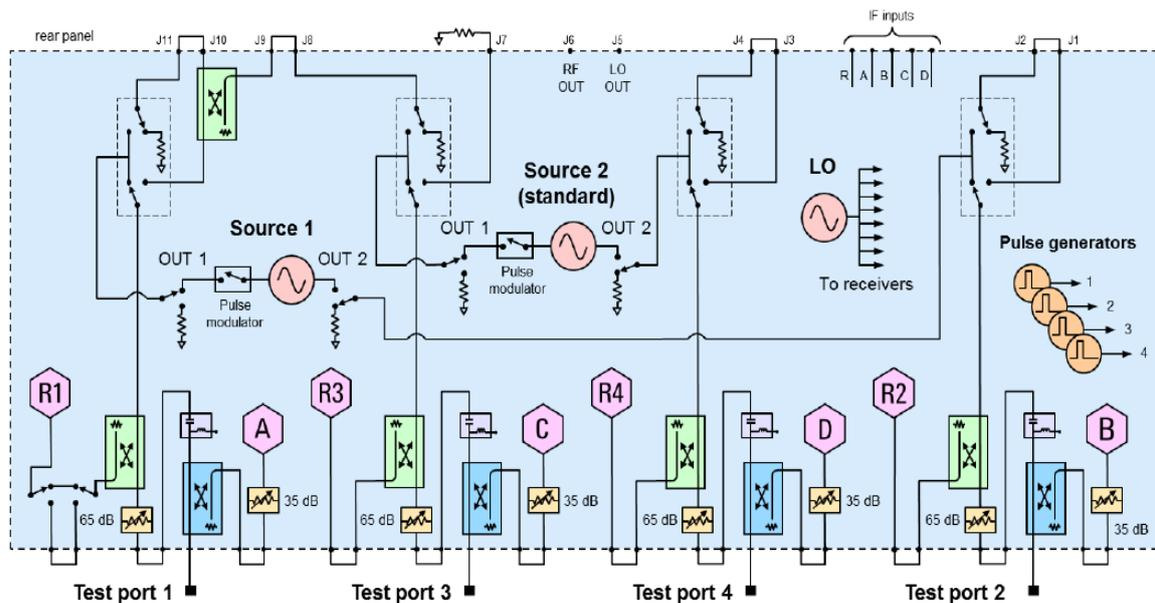
**Figure 4.2 - Agilent PNA-X N5242A Block Diagram**
