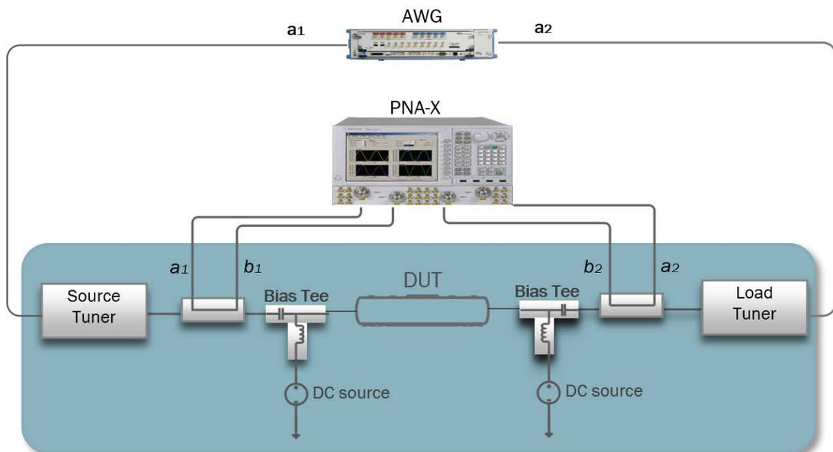
Figure 4.1- Characterization Setup Block Diagram
