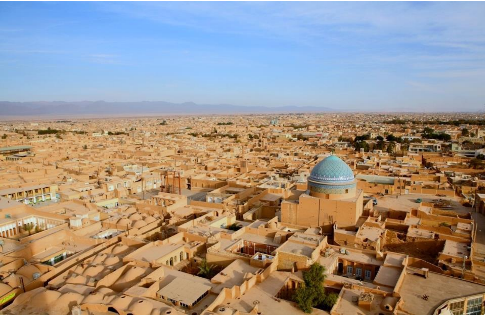
Figure 42. Compact, connected and continuous urban fabric of Yazd; a response to the harsh climate condition
