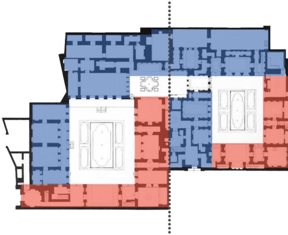
Figure 14. Summer and winter rooms and suites in Glosan house; winter suites are illustrated by blue and summer rooms are shown by red, illustration by author
