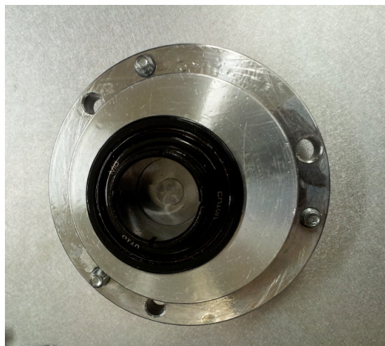
Figure 4.3: Eccentric Mounting Hub for Studying Backlash
