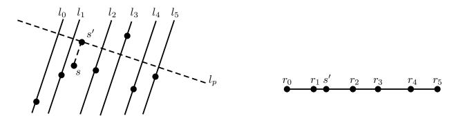
Figure 4.1: The left figure is an example of the Line/Point FTP with an active robot at points s, where  $l_p$  (shown in dashed) is the base for the corresponding 1-D FTP instance. The right figure is the corresponding 1-D FTP instance with the active robot s'.
