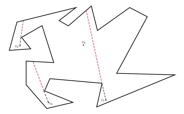
Figure 2.2: The Visibility Freeze-Tag Problem where only the initial robot can awaken others can be modelled as a Touring Polygons Problem. In the example shown here,  $v_0$  has to visit the dashed red lines to see  $v_1, v_2$  and  $v_3$ .
