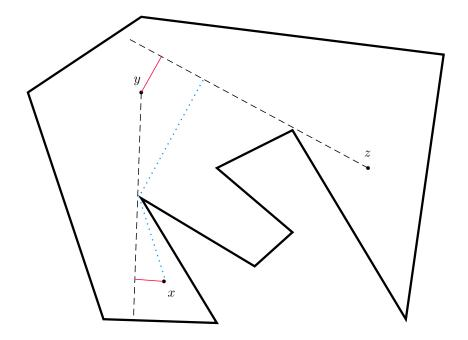
Figure 3.5: The shortest path for robot x to see z without intermediate robots (shown in dotted blue) is much longer than the shortest path (shown in solid red) with the help of the intermediate robot y.
