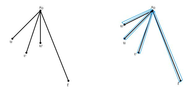
Figure 3.6: An example explaining the awakening strategy: We first sort all the children of  $s_0 - (u, v, w, t)$  based on the edge weights in ascending order (w, u, v, t). Once  $s_0$  is active,  $s_0$  will first unfreeze w, then move back to its original position. After that,  $s_0$  will move to unfreeze u, and then move back. The awakening procedure for v and t is similar.
