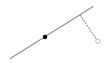
Figure 1.1: An example of the Line/Point FTP. In order to wake up the robot positioned at the solid circle, the shortest path for the robot at the empty circle is to move along the dashed line.
