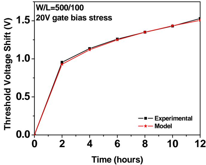
Figure 4.13.  $V_T$  shift as a function of stress time for a 12-hour, 20 V constant voltage stress test.
