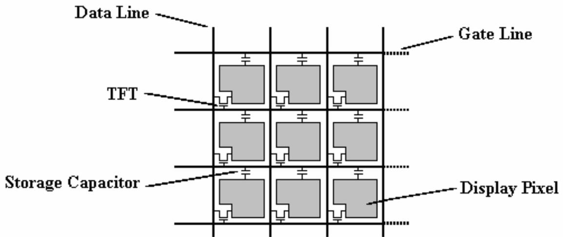
Figure 1.2. Schematic of pixel array of an AMLCD with TFTs used as switches.
