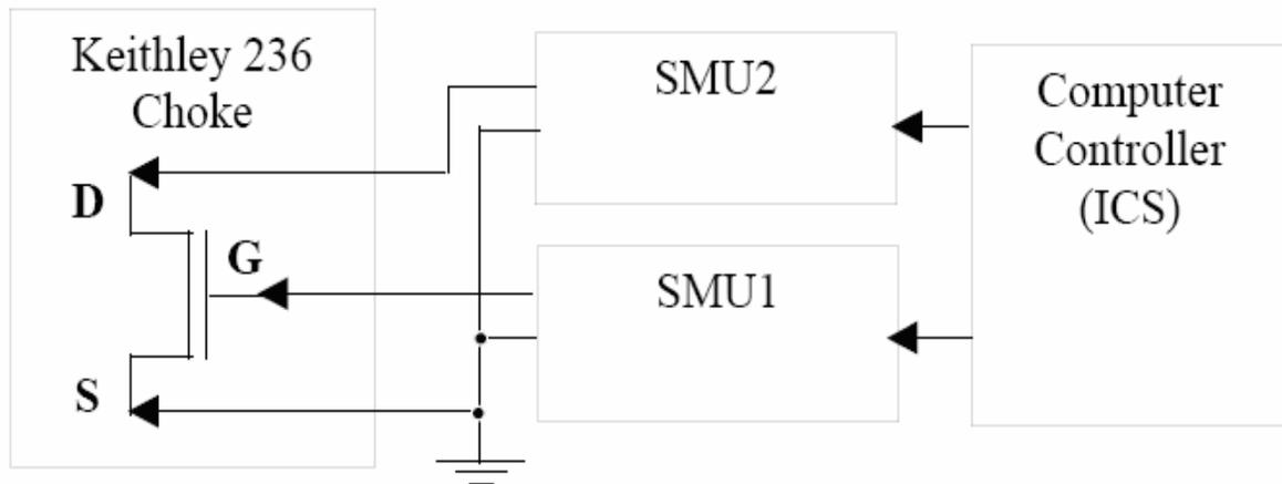
Figure 4.1. Experimental setup for TFT measurements using SMUs.
