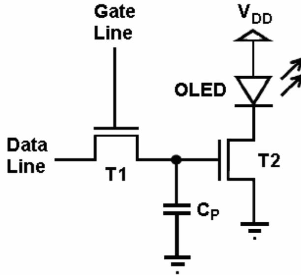
Figure 4.9. Schematic of a simple AMOLED pixel drive.
