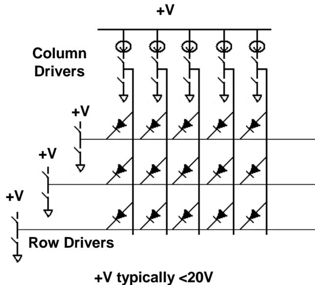
Figure 1.3. External control view of a PMOLED.
