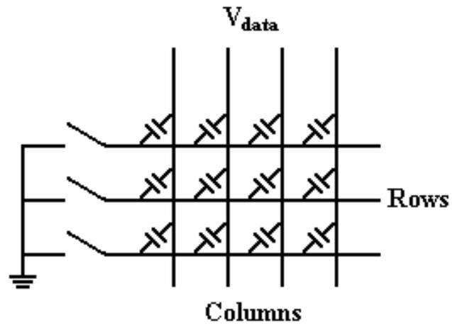
Figure 1.1. Schematic of pixel array of a PMLCD.
