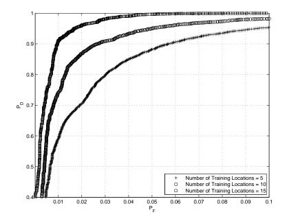
Figure 4.1: ROC curves of LFDA based scheme under different number of training locations
