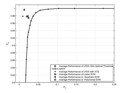
Figure 4.8: Comparison between SVM based schemes and LFDA based scheme in terms of  $P_D$  and  $P_F$
