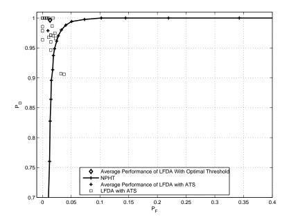
Figure 4.6: ROC curves of NPHT and LFDA based schemes with optimal threshold and with ATS
