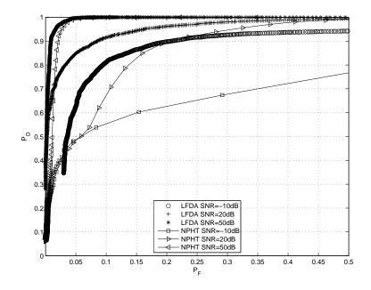
Figure 4.5: ROC curves of LFDA based scheme and NPHT under different SNRs
