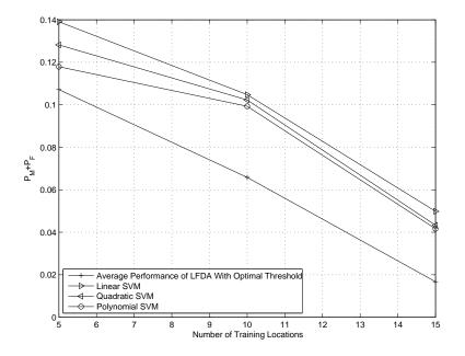
Figure 4.4: Comparison between SVM based schemes and LFDA based scheme in terms of  ${\cal P}_M + {\cal P}_F$
