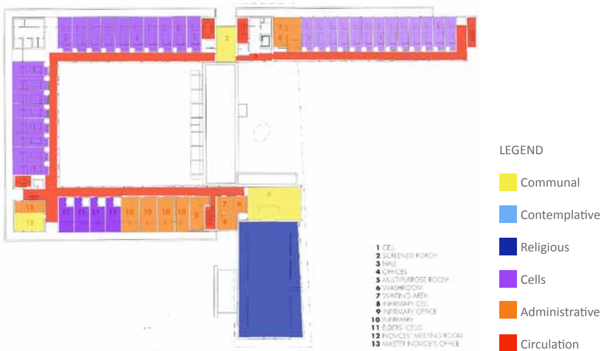
^ Fig. 13.5 - Ground floor plan of Abbaye Val Notre Dame, showing program distribution and circulation ^ Fig. 13.6 - Second floor plan of Abbaye Val Notre Dame, showing program distribution and circulation
