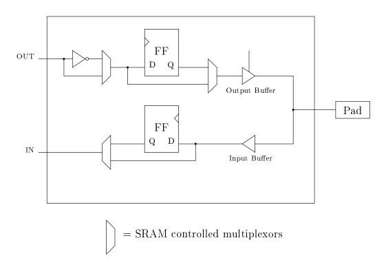
Figure 2.2: Functionality of an IOB
