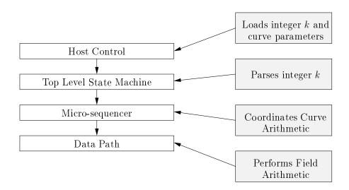
Figure 4.1: Co-Processor's Hierarchical Control Path
