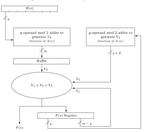
Figure 3.6: Modified Multiplier Data-Path
