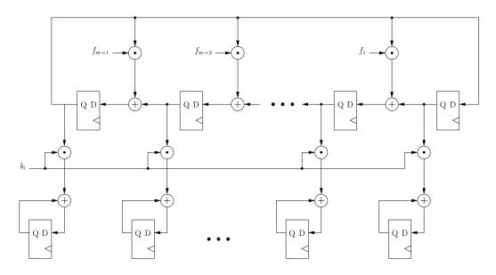
Figure 3.1: LFSR Based Multiplier
