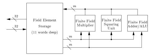
Figure 4.2: Co-Processor Data-Path
