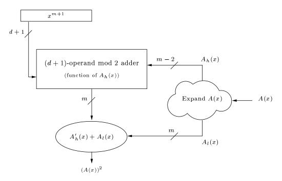
The prototype of this squaring unit for field  $GF(2^{163})$  using the NIST reduction
