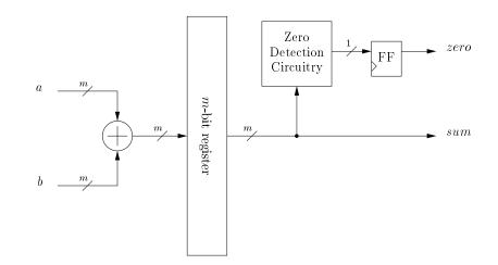
Figure 3.8: Data-Path of the Comparator/Adder
