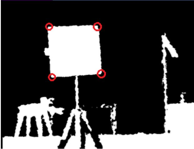
**Figure 3.1. Kinect depth image of calibration scene.** 3D-coordinates of the corners of the rectangular object (circled) were manually using the Microsoft Kinect SDK and used to transform Kinect coordinate system into the control coordinate system.
