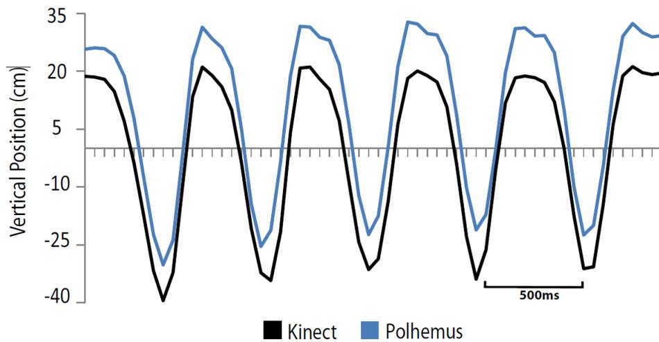
**Figure 3.8. Temporal resolution of Kinect compared to the gold standard system.** Event shown is the calibration movement consisting of rapid elbow flexion and extension cycles performed prior to each task. The two lines depicted above are the vertical positions of the Kinect hand virtual marker (blue) and the gold standard ulnar styloid marker (black).
