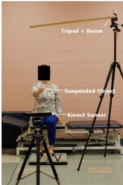
**Figure 4.1. Experimental setup for study two.** The Kinect sensor is positioned to project on the participant frontally. The tripod and boom setup is used to suspend an object via fine-gauge wire to ensure that there are no external objects occluding the participant from the Kinect sensor.
