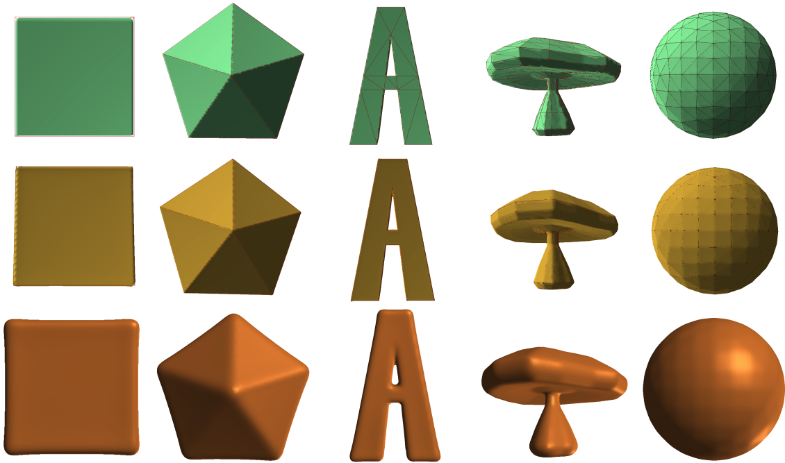
Figure 6.5: 3D approximating reconstruction. First Row: interpolation results; Second Row: approximation results with \epsilon = 0.02 . Last Row: approximation results with \epsilon = 0.02 and h = 0.08
