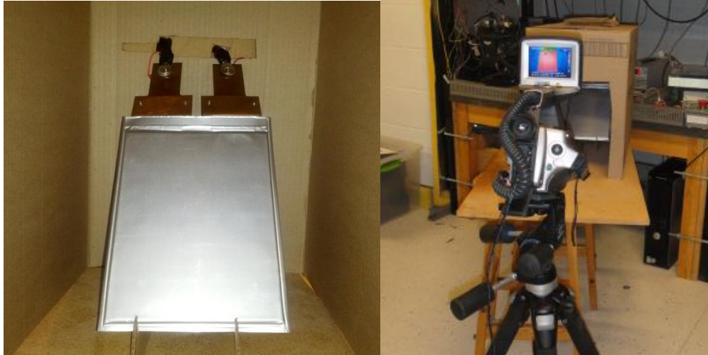
FIGURE 3.19: THERMO-GRAPHIC EXPERIMENTAL SET-UP SHOWING (L) BATTERY ON STAND AND (R) BATTERY AND CAMERA POSITIONING
