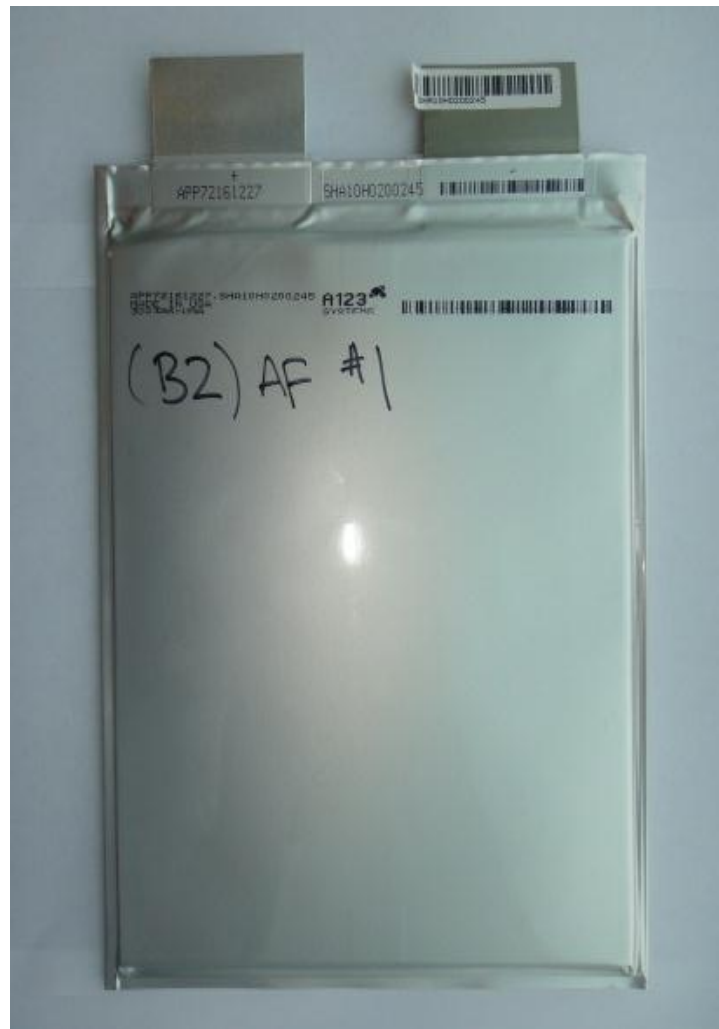
FIGURE 3.1: COMMERCIAL 20AH LiFePO 4 /GRAPHITE PRISMATIC BATTERY
