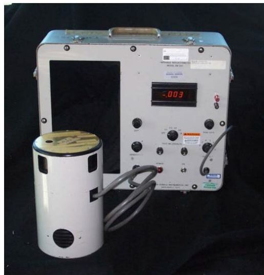
FIGURE 3.20: PHOTOGRAPH OF GIER-DUNKLE DB100 INFRA-RED REFLECTOMETER
