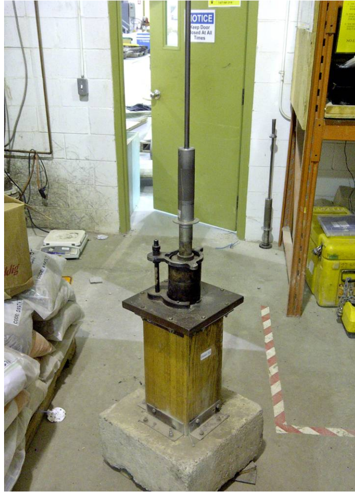
Figure 4.1 Marshall compaction hammer (LVM Toronto laboratory, 2013)
