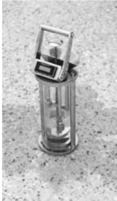
Figure 2.10 Typical Outflow Meter apparatus (National Driller, 2001)
