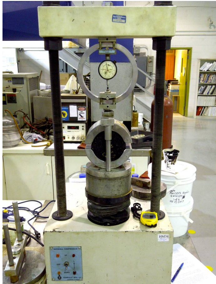
Figure 4.2 Marshall Stability machine (LVM Toronto laboratory, 2013)
