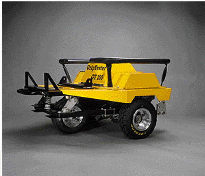
Figure 2.11 Typical GripTester ( Skid Resistance (Surface Friction) Tester, n.d. ).
