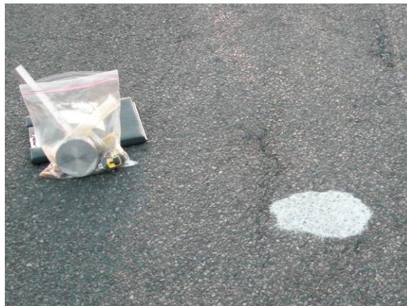
Figure 2.9 Sand Patch test (Field site visit, 2012)
