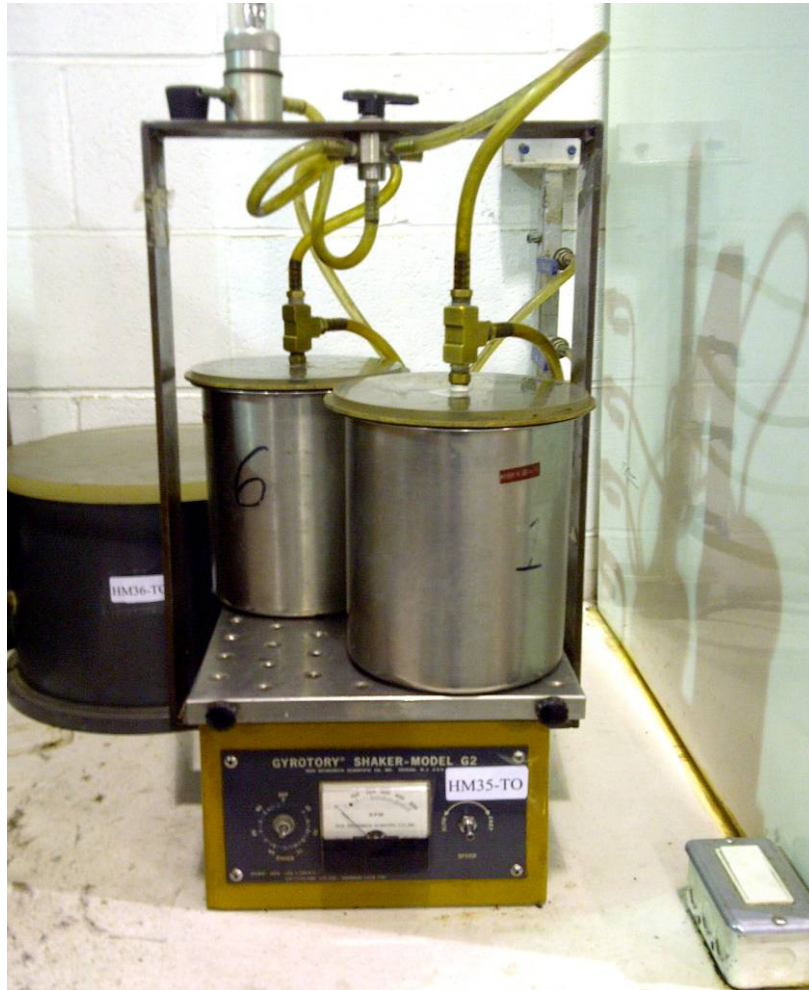
Figure 4.4 Maximum Relative Densometer tester (LVM Toronto laboratory, 2013)
