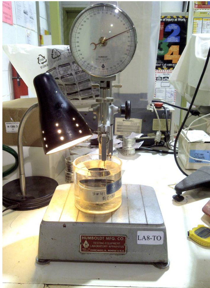
Figure 4.5 Penetration test equipment (LVM Toronto laboratory, 2013)
