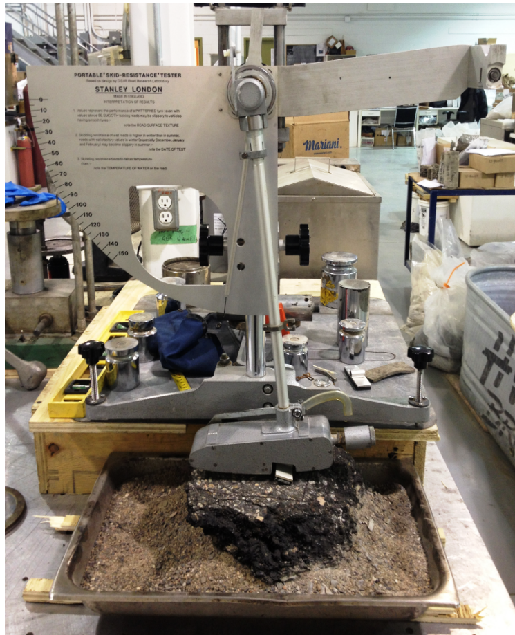
Figure 4.8 British Pendulum Tester (LVM Toronto laboratory, 2013)
