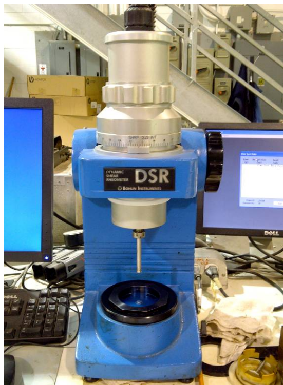
Figure 4.7 Dynamic Shear Rheometer (LVM Toronto laboratory, 2013)
