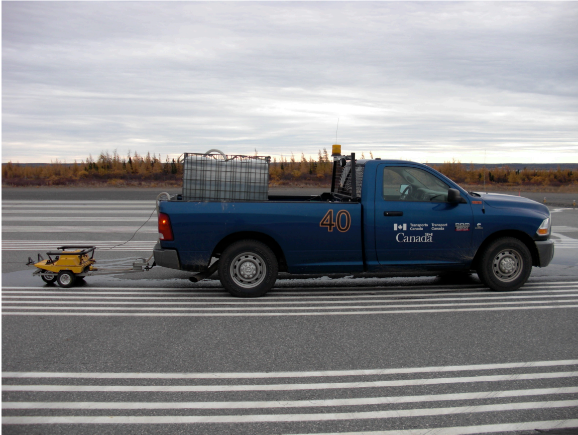
Figure 5.8 2013 GripTester operations (Field Testing, 2013)
