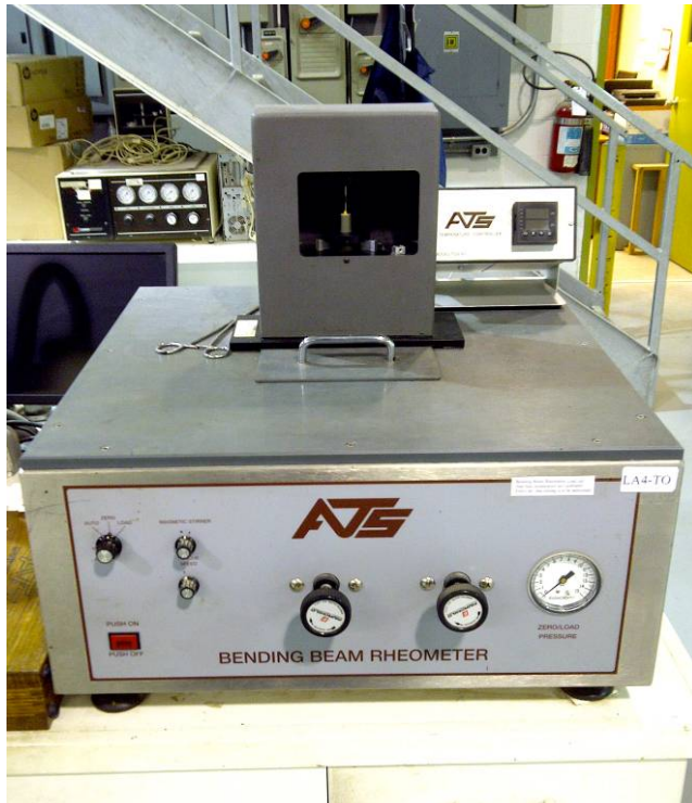
Figure 4.6 Bending Beam Rheometer (LVM Toronto laboratory, 2013)
