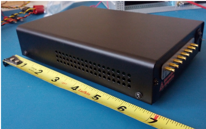
Figure B.3: Photograph of the X6-1000M board[16] plugged into the eInstrument[15]. Front connectors shown here are the SSMC variety.
