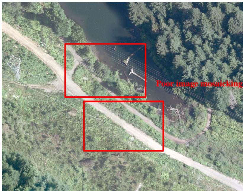
Figure 4.23 Poor image mosaicking quality of the orthophoto
