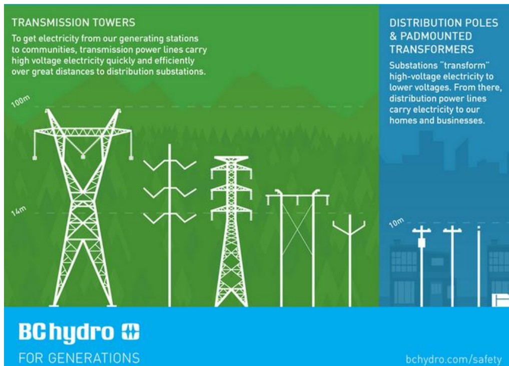
Figure 2.5 Types of different transmission towers in BC, Canada
