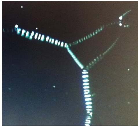
Figure-A16: A few dislocations in lamellar phase are observed between two crossed polarizers under an optical microscope. The dimension of the image is about 0.22mmx0.22mm.
