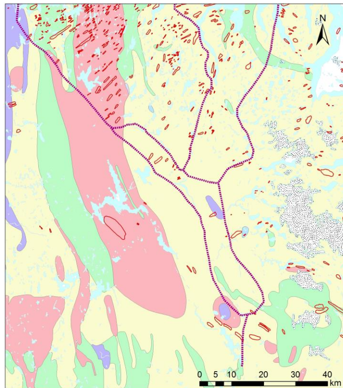
Figure 3-23: Streamlined hill polygons over bedrock geology map (See Figure 3-1 or Figure 3-22 for legend). In the north, the density of the streamlined hills is higher in the Cumberland Batholith than the Hall Block or the metasediments.
