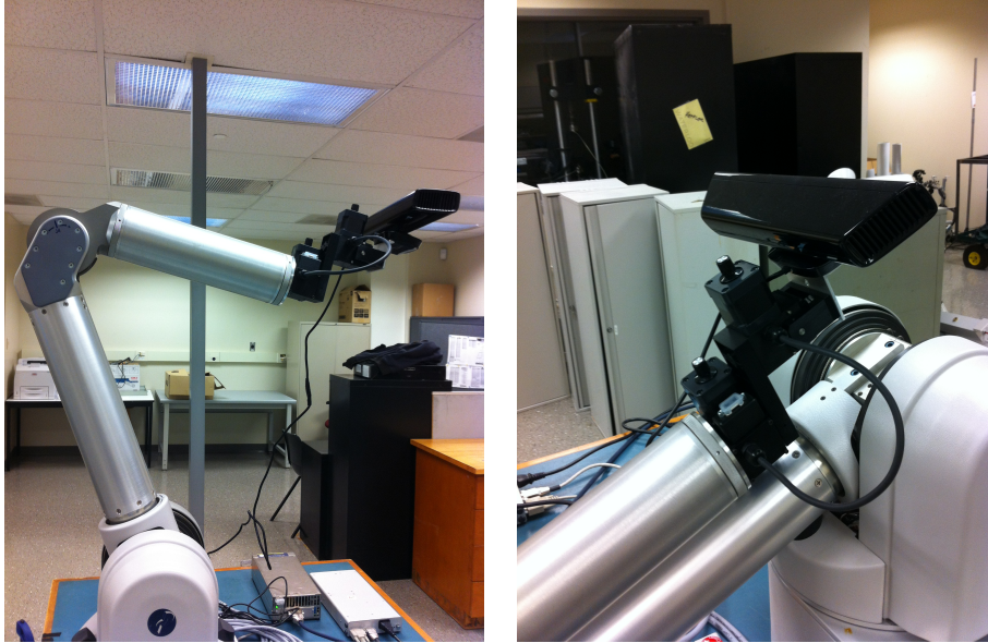
Figure 3.1: The Barrett WAM with the Kinect camera installed
