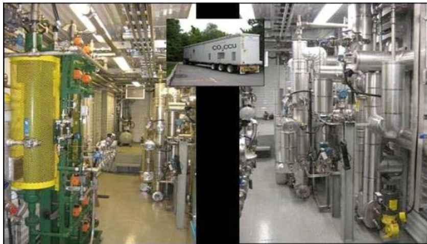
Figure 3.2 Trailer-mounted configuration of pilot-scale CanCO 2 (Zanganeh et al., 2009)
