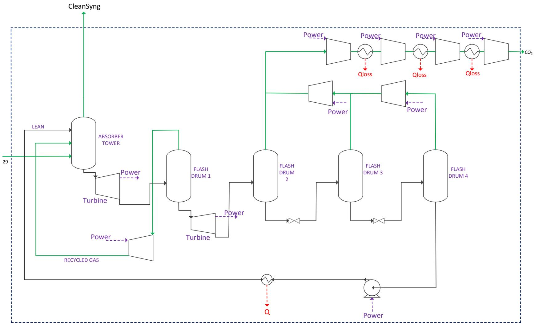
**Figure 2.6:** Flow diagram of CO<sub>2</sub> removal and capturing (Based on [51, 52])
