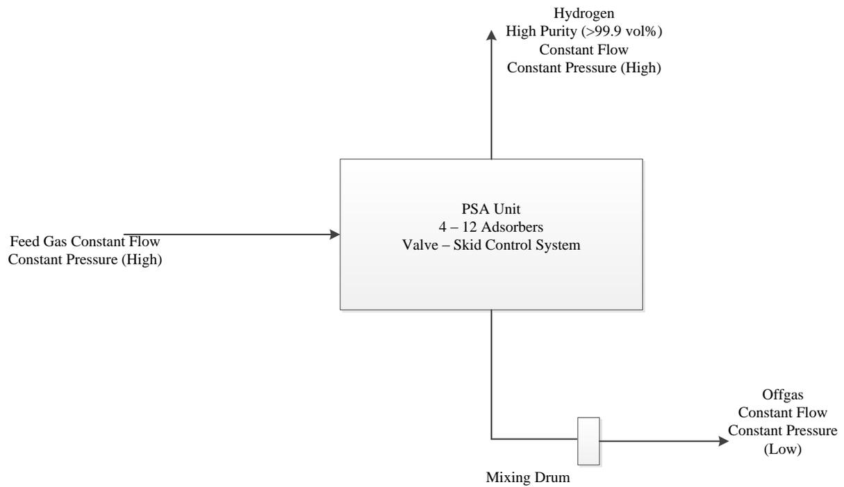
**Figure 2.7:** PSA basic flow schema (Adapted from [54])
