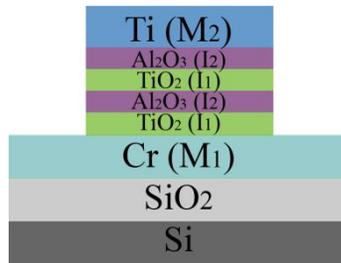
**Figure 5.2:** A schematic diagram of the MI<sup>4</sup>M diode
