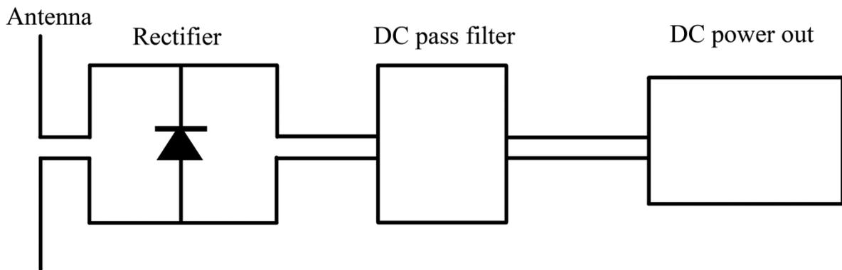
**Figure 1.1:** A block diagram of a rectenna
