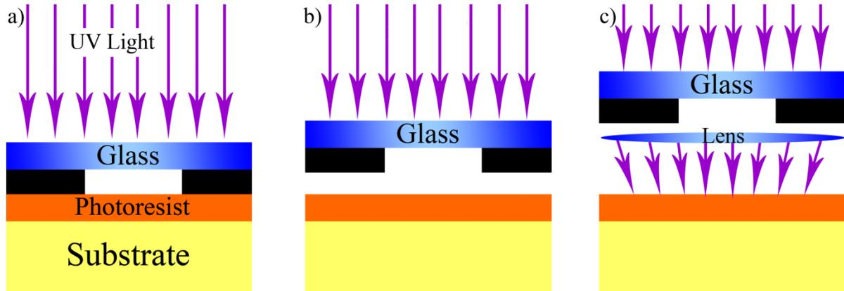
**Figure 3.2:** A schematic illustration of exposure methods in photolithography: a) contact printing, b) proximity printing, c) projection printing
