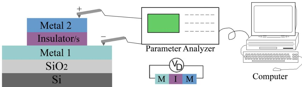
**Figure 6.1:** A schematic diagram of Semiconductor Characterization System
