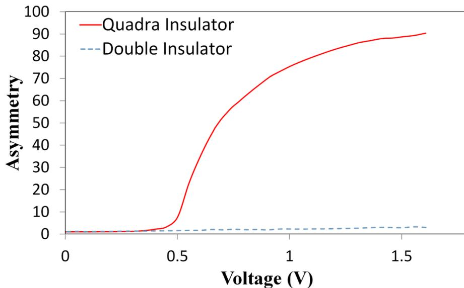
**Figure 6.5:** Asymmetry of MI<sup>2</sup>M and MI<sup>4</sup>M diodes
