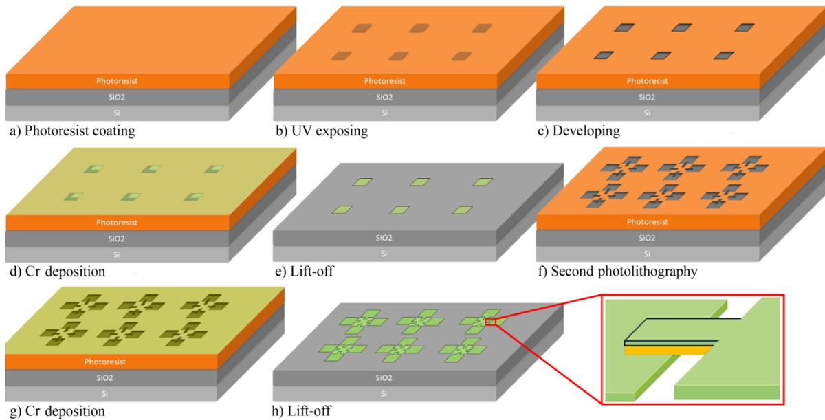
**Figure 4.3:** Fabrication steps of Cr/Al<sub>2</sub>O<sub>3</sub>/Cr MIM diode
