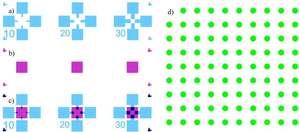
**Figure 4.1:** a) Mask A, b) Mask B, c) Combination of Mask A and MaskB2, d) Mask C.
