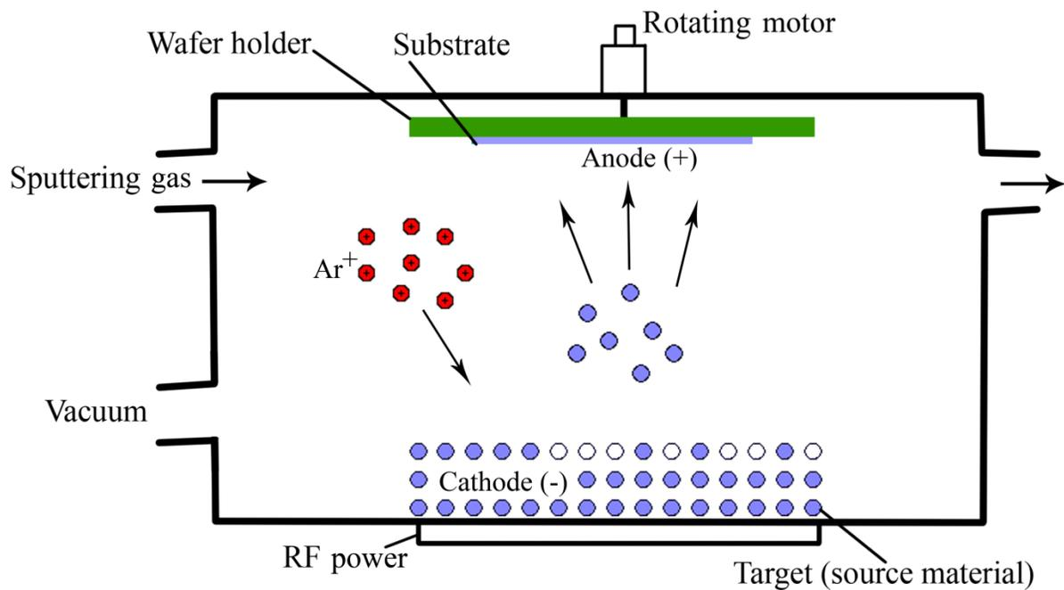
**Figure 3.7:** A schematic diagram of sputtering mechanism
