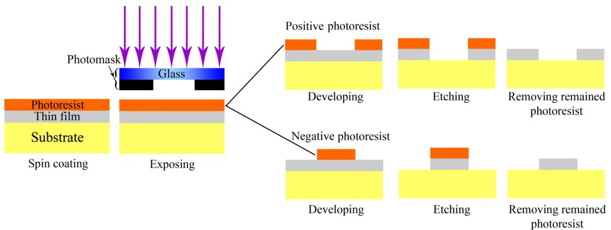
**Figure 3.3:** A Schematic illustration of the photolithography process with positive and negative photoresists
