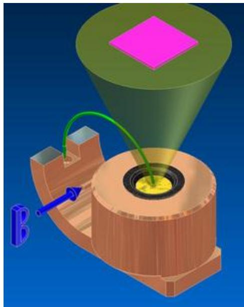
**Figure 3.5:** A schematic illustration of the e-beam evaporation mechanism [24]
