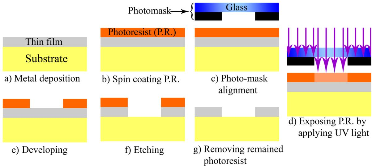
**Figure 3.1:** Basic processing steps to fabricate metal patterns on a substrate
