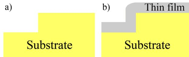
**Figure 3.8:** A schematic diagram of sputtering deposition on a stepped substrate
