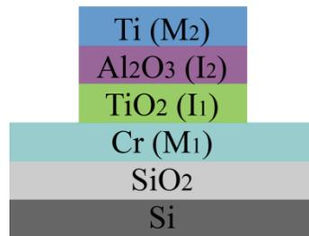
**Figure 5.1:** A schematic diagram of the MI<sup>2</sup>M diode
