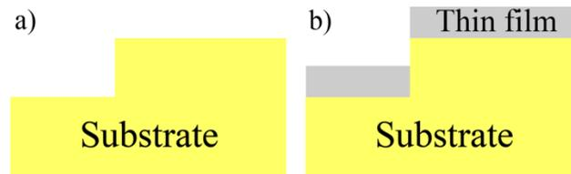
**Figure 3.6:** A schematic diagram of e-beam deposition on a stepped substrate
