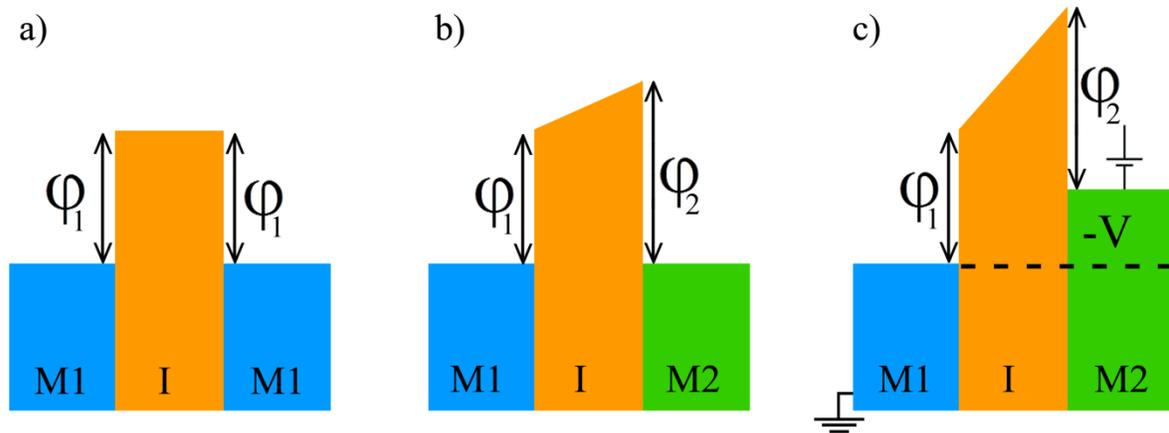
**Figure 2.1:** Energy Band Diagram of a MIM diode when (a) two metals are the same, (b) metal 1 and metal 2 is different, (c) negative voltage applied to metal 2
