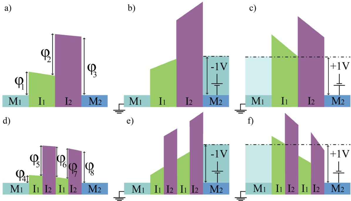
**Figure 5.3:** Energy band diagram of the  $MI^2M$  diode: a) no bias applied; b) negative; c) positive bias applied to Ti. Energy band diagram of the  $MI^4M$  diode: d) no bias applied; e) negative; f) positive bias applied to Ti.
