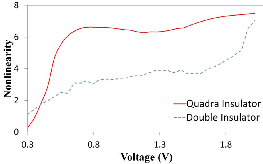
**Figure 6.6:** Nonlinearity of MI<sup>2</sup>M and MI<sup>4</sup>M diodes
