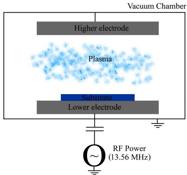
**Figure 3.10:** A schematic representation of RIE
