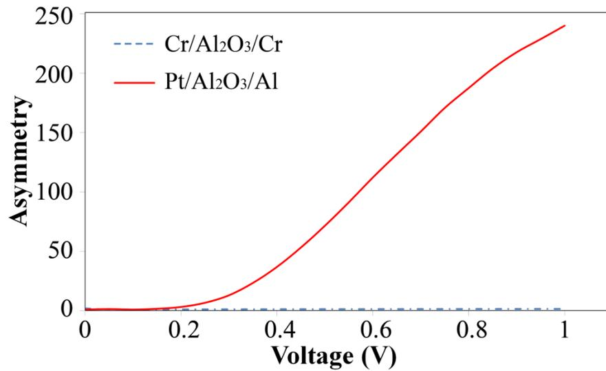
**Figure 6.3:** Asymmetry curves of Cr/Al<sub>2</sub>O<sub>3</sub>/Cr and Pt/Al<sub>2</sub>O<sub>3</sub>/Al MIM diodes
