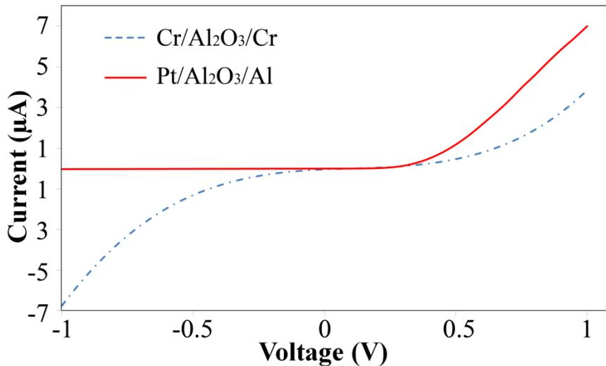
**Figure 6.2:** I-V curves of Cr/Al<sub>2</sub>O<sub>3</sub>/Cr and Pt/Al<sub>2</sub>O<sub>3</sub>/Al MIM diodes
