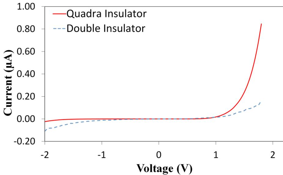
**Figure 6.4:** I-V curve of MI<sup>2</sup>M and MI<sup>4</sup>M diodes
