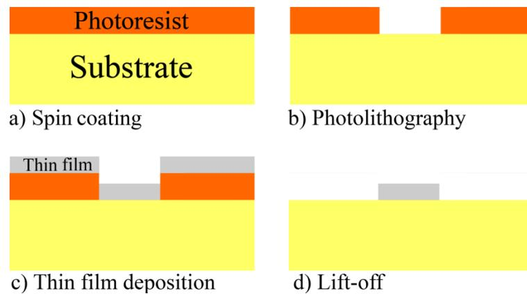
**Figure 3.11:** A schematic representation of the lift-off process
