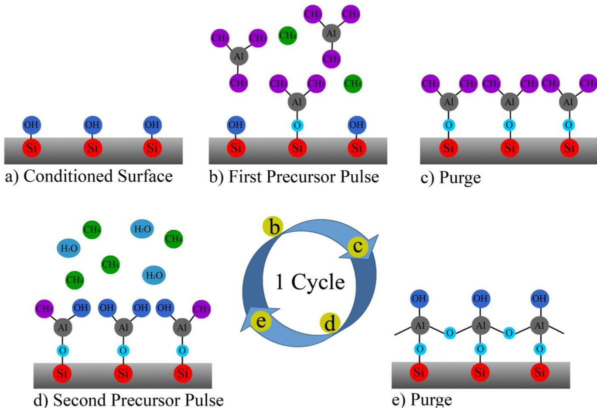
**Figure 3.9:** A schematic representation of one ALD cycle [25]
