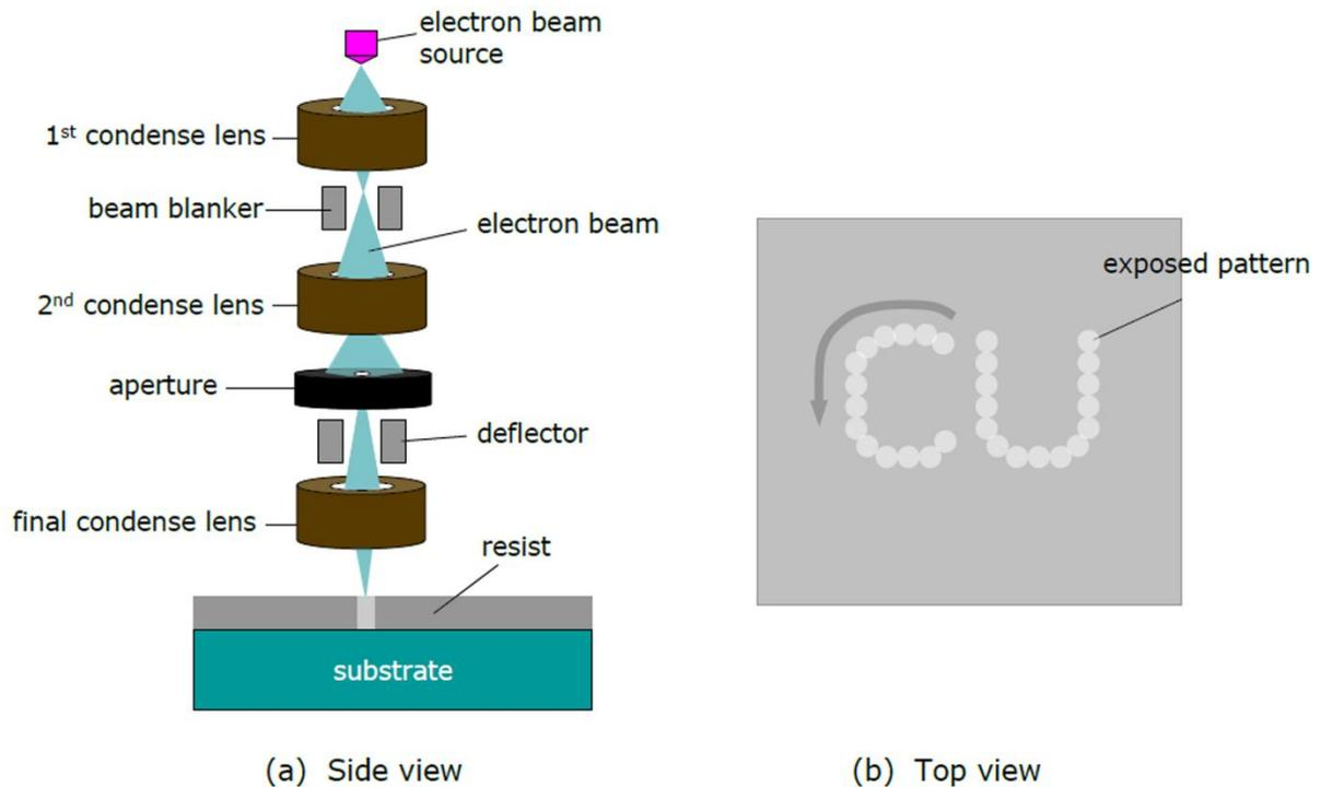
**Figure 3.4:** A Schematic diagram of e-beam lithography. The e-beam is focused on a resist to generate patterns by exposing dot by dot: (a) side view of the e-beam lithography setup; (b) top view of the exposed pattern by a serial writing [20].
