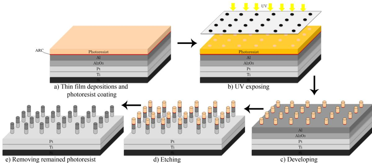
**Figure 4.2:** Fabrication steps of Pt/Al<sub>2</sub>O<sub>3</sub>/Al MIM diode
