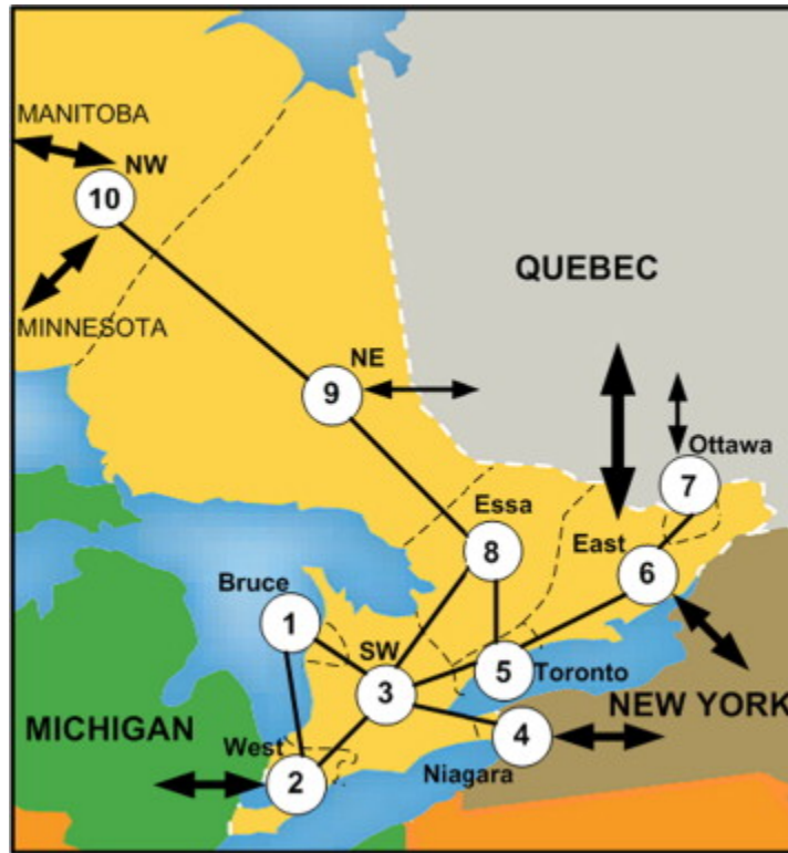
Figure 3.3 Ontario's power grid and its transmission zones [73]
