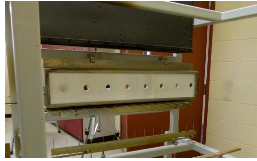
Figure 4.12 Photograph of IMO LIFT device radiant heater and sample holder
