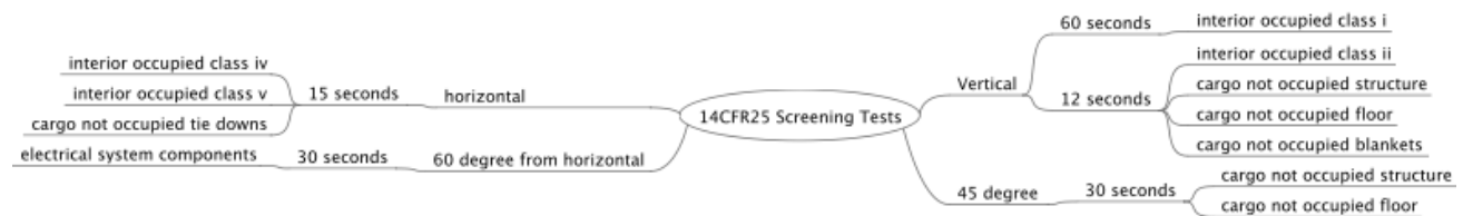
Figure 4.7 Summary of flame spread screening tests from 14 CFR 25 Appendix F, Part 1
