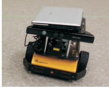
Figure 2.1: Photograph of the differential drive robot Chameleon R200.
