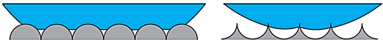
Figure 29: Different surface profiles showing the different kurtosis values for a surface, where the more positive the value (shifted towards the profile on the right), the more a surface will show hydrophobic and icephobic tendencies [67]
