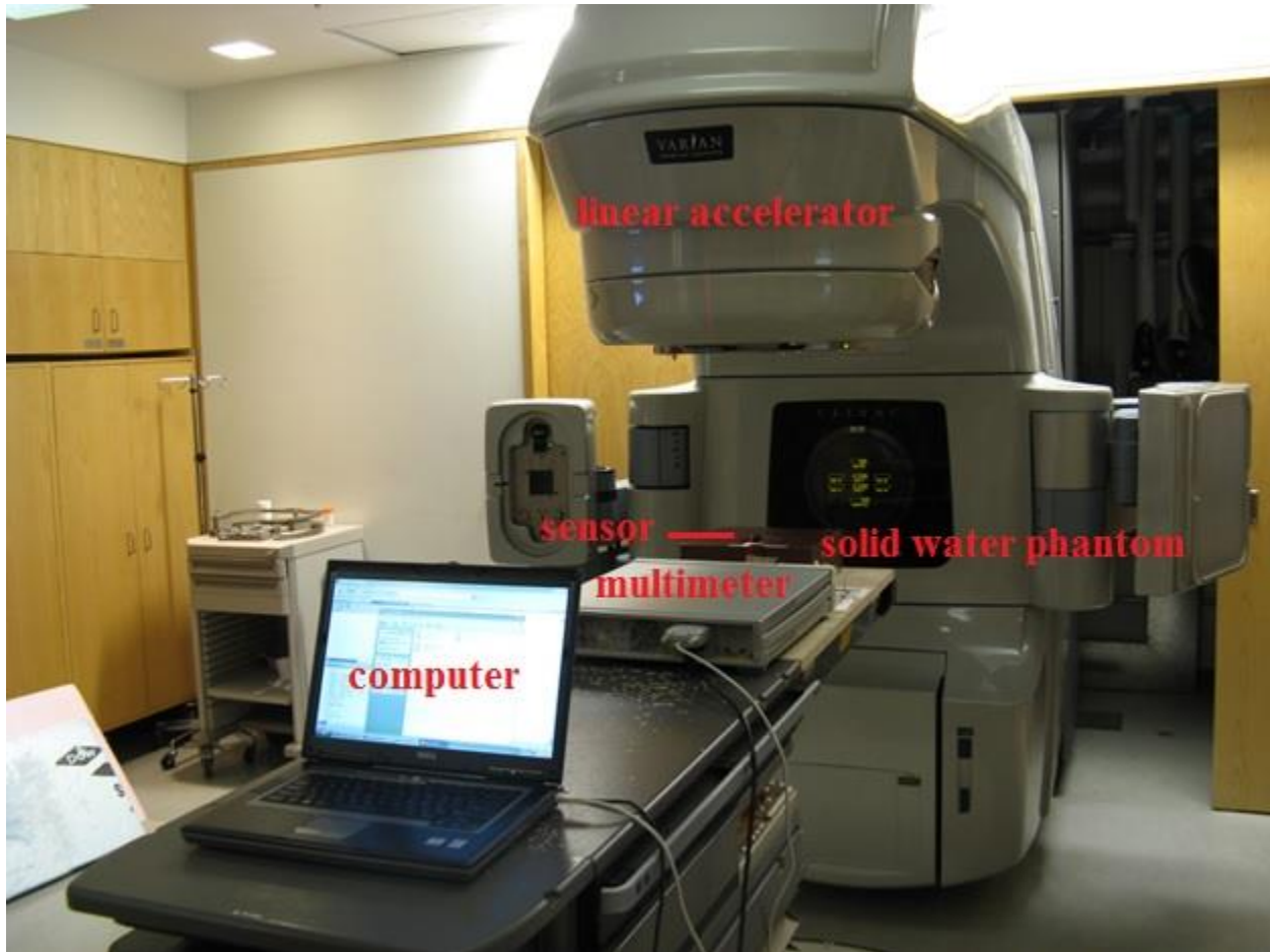
Figure 4.1 Varian linear accelerator in Grand River Cancer Centre, Kitchener, Ontario. This machine has been used as an X-ray source for characterization of the fabricated sensors.
