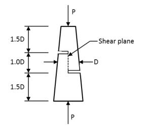
Figure 1.1 Non-dimensional configuration of shear test pole stub specimen
