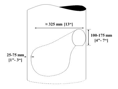
Figure 2.9 Range of nesting damage dimensions observed by Hydro One [4]
