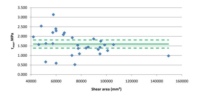
Figure 3.10 Variation of measured shear strength versus gross shear area
