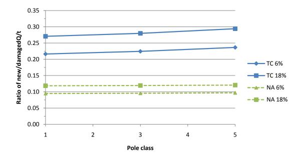
Figure 5.19 Effect of nesting damage on statical moment of area for different pole class with the shell thickness determined based on a percentage of the cross-section diameter
