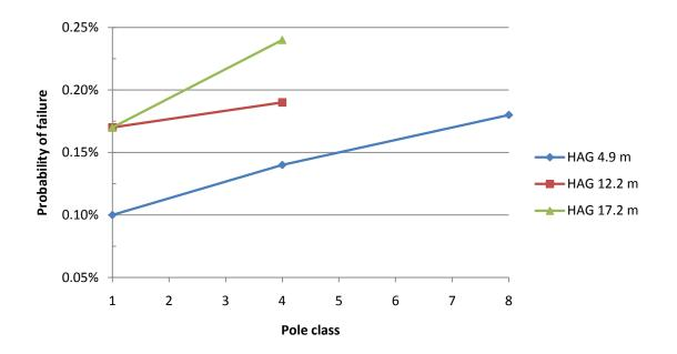
Figure 5.6 Variation of probability of failure versus pole class for different pole heights (wind only)
