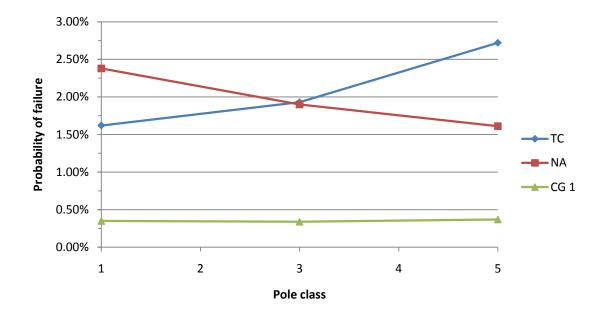
Figure 5.15 Overall probability of failure for poles with nesting damage
