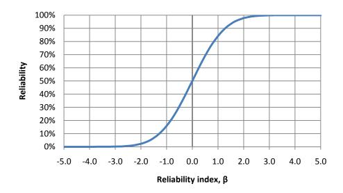
Figure 2.6 Relationship of reliability and reliability index based on normal distribution
