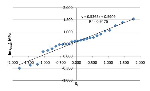
Figure 3.14 Probability paper plot for shear strength following a log-normal distribution
