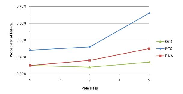
Figure 5.13 Probability of failure for poles with feeding damage
