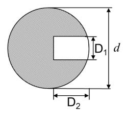
Figure D.5 Exploratory and feeding damage oriented with the neutral axis
