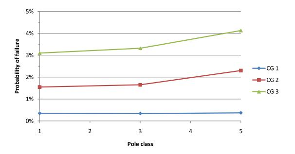
Figure 5.9 Variation of probability of failure for poles of different classes and construction grades
