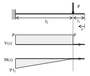
Figure B.2 Point load on cantilevered structural member
