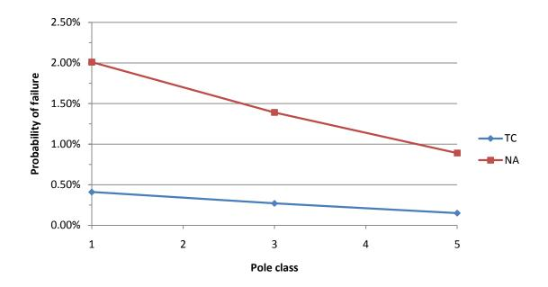
Figure 5.18 Probability of shear failure for poles with nesting damage
