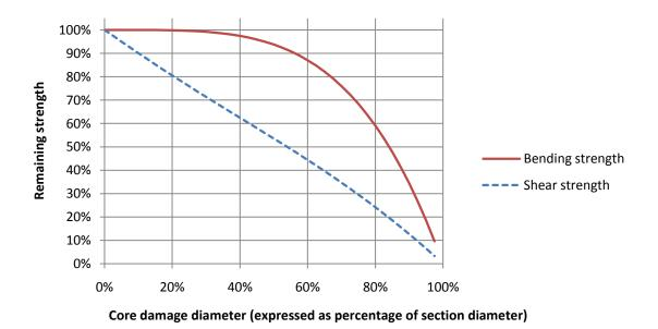
Figure 5.11 Decrease in strength in circular section due to section core loss
