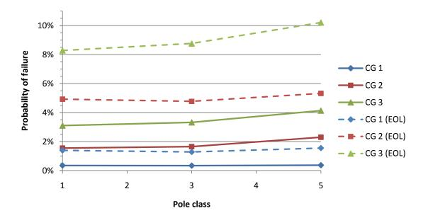
Figure 5.10 Comparison of probability of failure for as-new and end-of-life Red Pine wood poles
