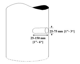
Figure 2.7 Range exploratory damage dimensions observed by Hydro One [4]
