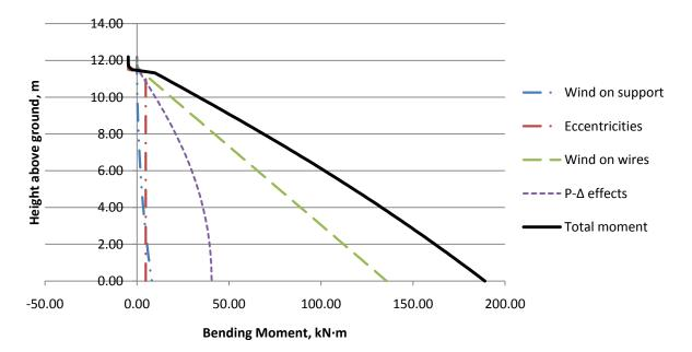
Figure 5.1 Contribution of different loads to total bending moment
