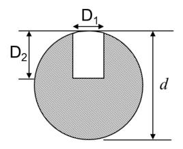
Figure D.1 Idealized cross-section at location of exploratory and feeding damage
