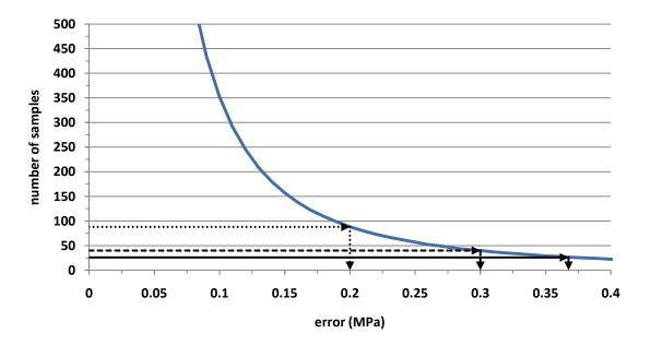
Figure 3.12 Selection of sample size based on target 95 % confidence error
