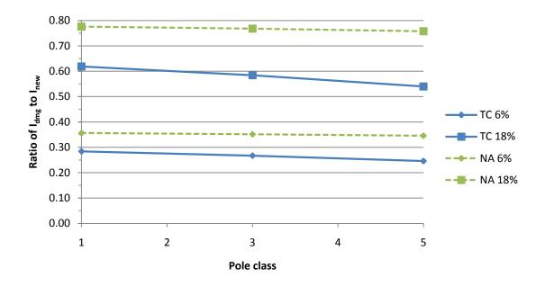
Figure 5.17 Effect of nesting damage on moment of inertia for different pole classes with the shell thickness determined based on a percentage of the cross-section diameter
