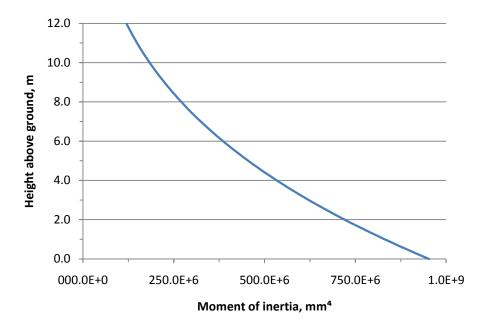
Figure 5.3 Variation of moment of inertia along the pole height
