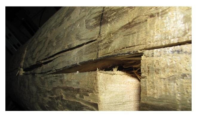
Figure 3.7 Failed specimen with strut and two separate failure planes
