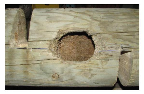
Figure 3.9 Untested specimen with woodpecker damage
