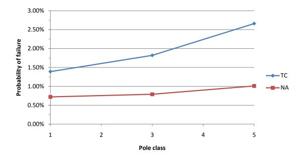
Figure 5.16 Probability of bending failure for poles with nesting damage
