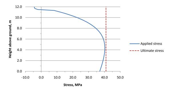
Figure 5.2 Variation of flexural stress along the pole height
