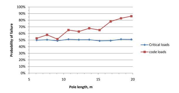
Figure 5.4 Level 2 analysis comparison between Class 2 poles loaded with code-specified horizontal load and calculated critical load
