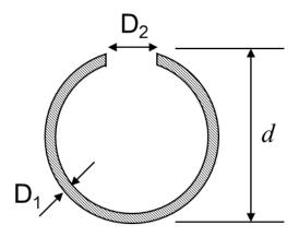
Figure D.3 Idealized cross-section at location of nesting damage
