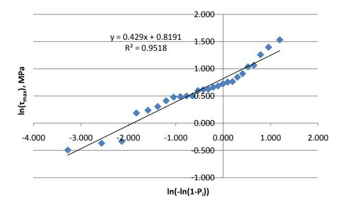
Figure 3.15 Probability paper plot for shear strength following a Weibull distribution
