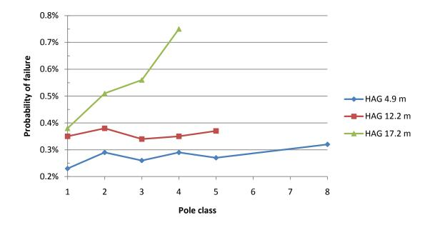
Figure 5.7 Variation of probability of failure versus pole class for different pole heights (wind on ice)
