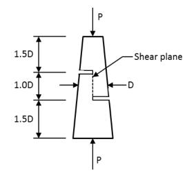
Figure 3.2 Non-dimensional specimen configuration for full-size pole shear strength testing
