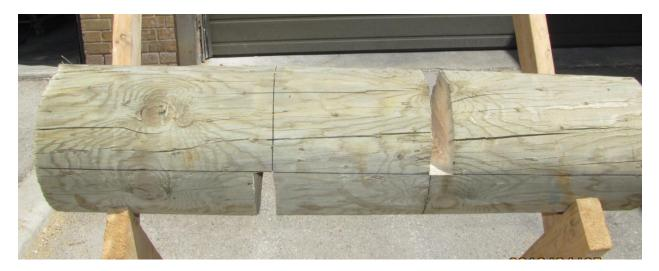
Figure 3.3 Typical specimen used to determine full-size pole shear strength
