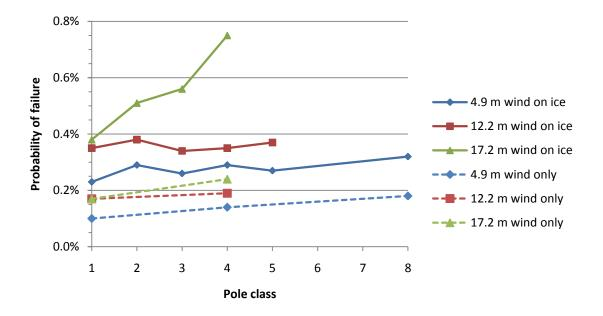
Figure 5.8 Comparison between wind-only and wind-on-ice loading
