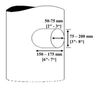
Figure 2.8 Range of feeding damage dimensions observed by Hydro One [4]
