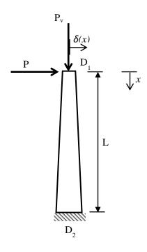
Figure 2.2 Cantilevered non-prismatic member
