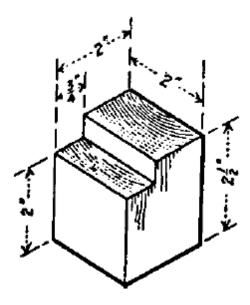
Figure 3.1 Test specimen configuration for shear-parallel-to-grain measurement (ASTM D143-09)
