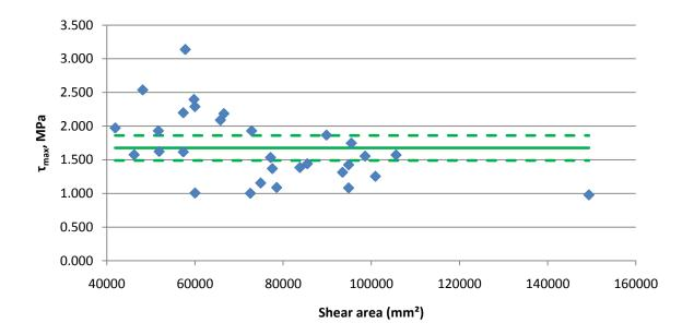
Figure 3.11 Variation of measured shear strength versus net shear area
