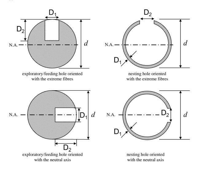
Figure 4.1 Assumed shapes and orientations of woodpecker damage
