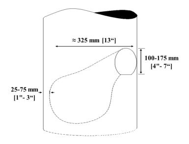
Figure 5.14 Typical nesting damage hole dimensions
