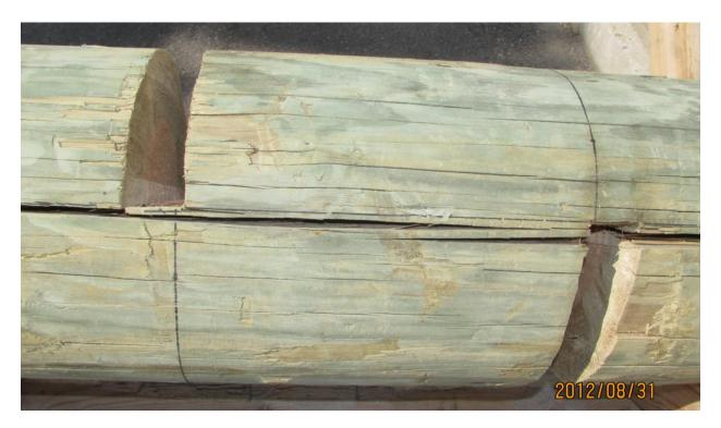
Figure 3.8 Untested specimen with deep check
