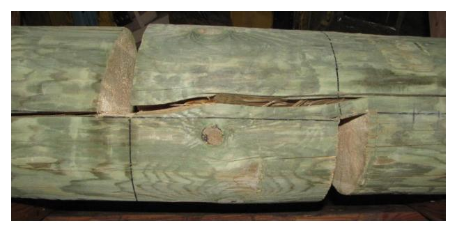
Figure 3.6 Failed specimen with strut formed at one end
