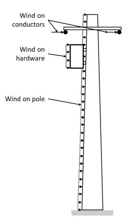
Figure 2.1 Wind forces acting on a typical wood utility pole
