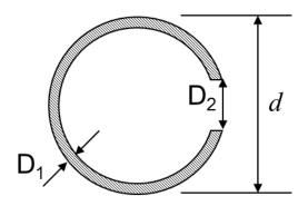
Figure D.6 Nesting damage oriented with the neutral axis
