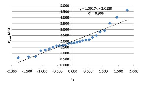
Figure 3.13 Probability paper plot for shear strength following a normal distribution
