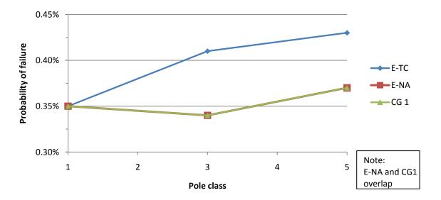
Figure 5.12 Probability of failure for poles with exploratory damage
