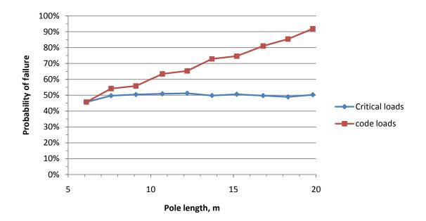
Figure 5.5 Level 2 analysis comparison between Class 4 poles loaded with code-specified horizontal load and calculated critical load
