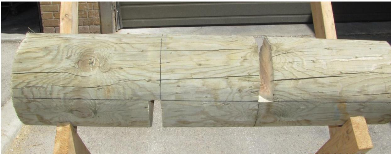
Figure 3.3 Typical specimen used to determine full-size pole shear strength
