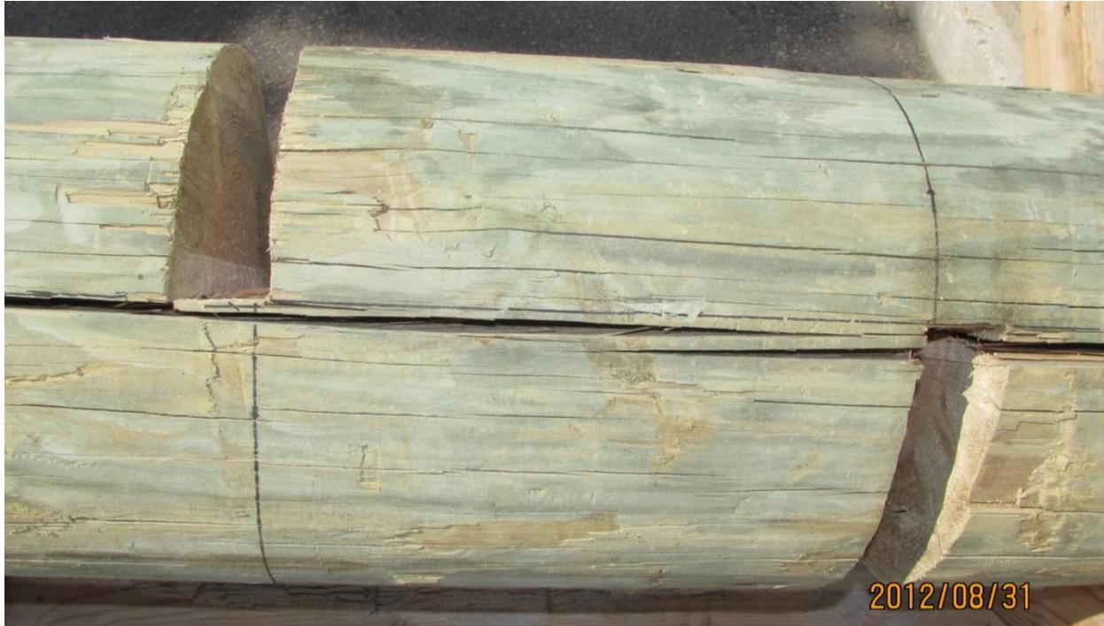
Figure 3.8 Untested specimen with deep check
