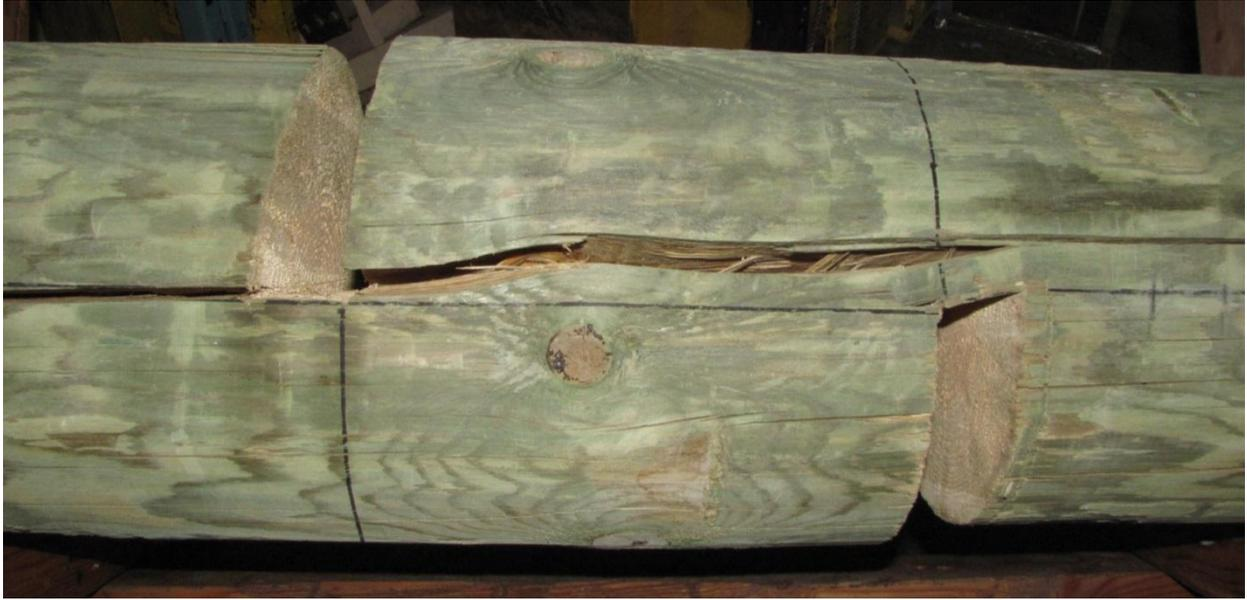
Figure 3.6 Failed specimen with strut formed at one end
